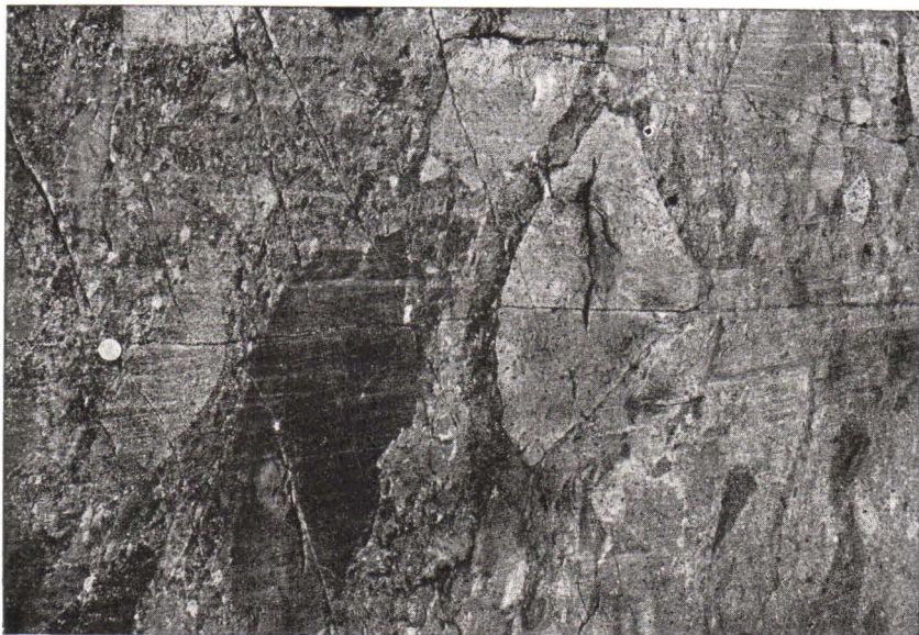
Fig. 11. Agglomeratic metabasaltic tuff. Island of Stor-Brändholm in the Pellinge area, south Finland. 1 : 7.
