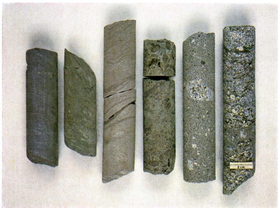
Fig. 8. Drill cores of the Söderfjärden rock types (from left to right): shale, siltstone, sandstone, conglomerate, tuffaceous breccia, altered Vaasa granite.
