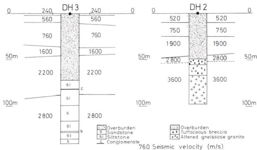
Fig. 7. Drilling results from drill holes 2 and 3
