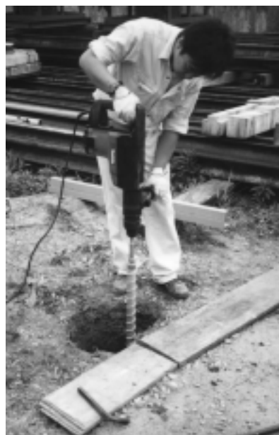
Figure. 8. Surface soil sampling with electric hand drill.
