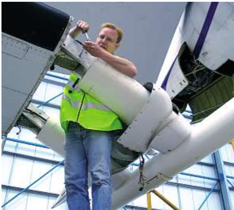
Fig. 6b. The EM pod fitting to the Twin Otter wing. Photo: Kai Nyman
