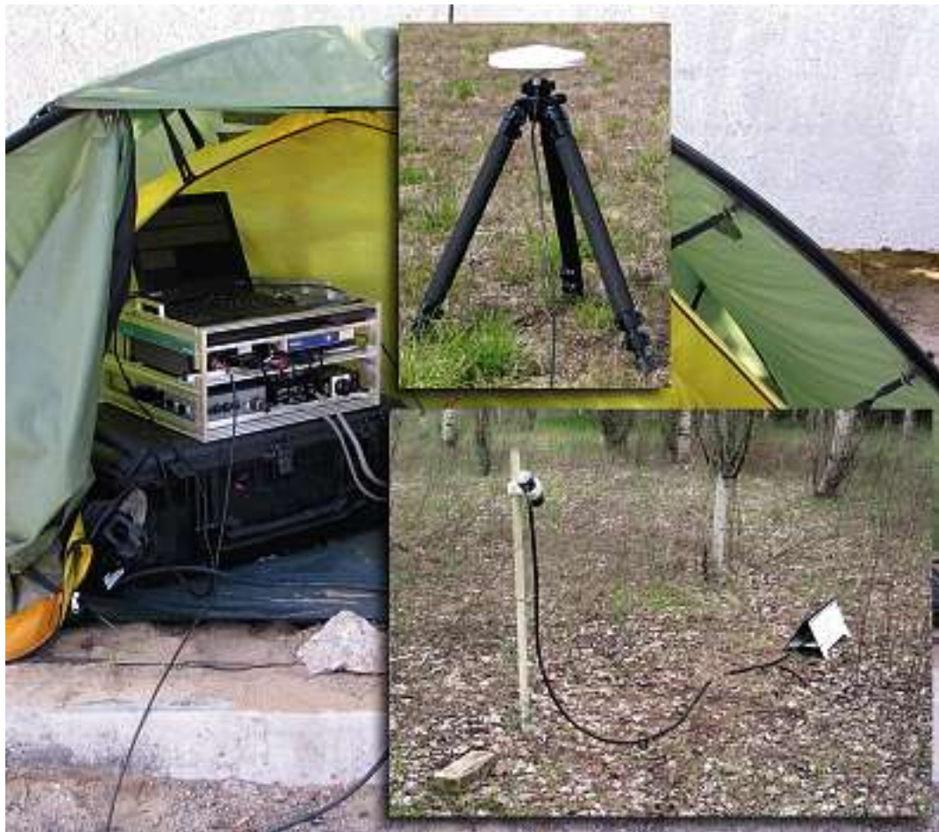
Fig. 12. Base station "housings". Magnetometer, GPS unit and control pc inside the tent, magnetometer sensor and GPS antenna in the field. Photo: Kai Nyman
