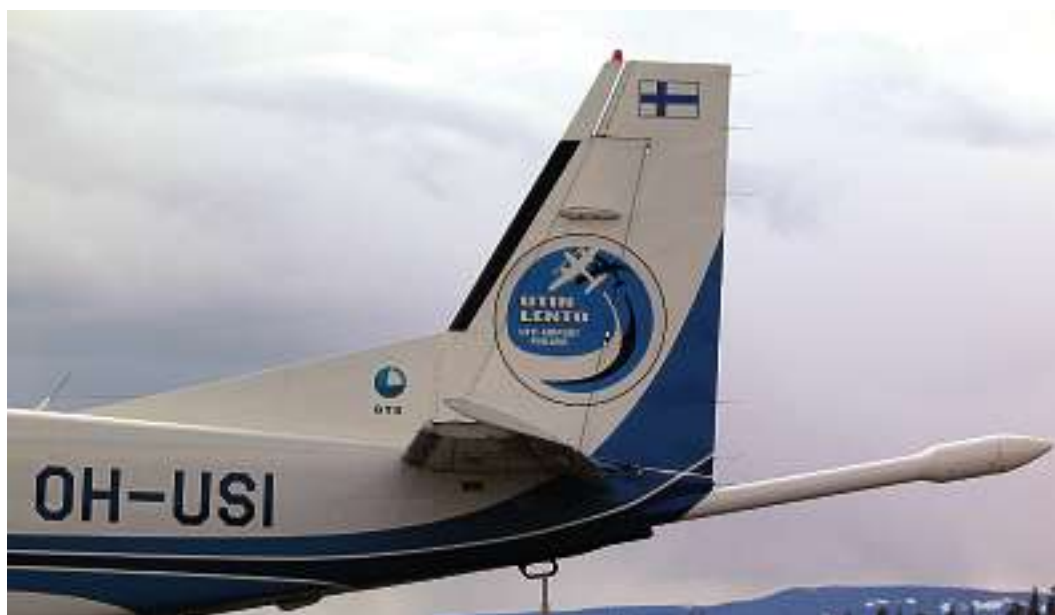
Fig. 8. Tail boom installation of the Cs magnetometer sensor in the Cessna Caravan. Photo: Kai Nyman
