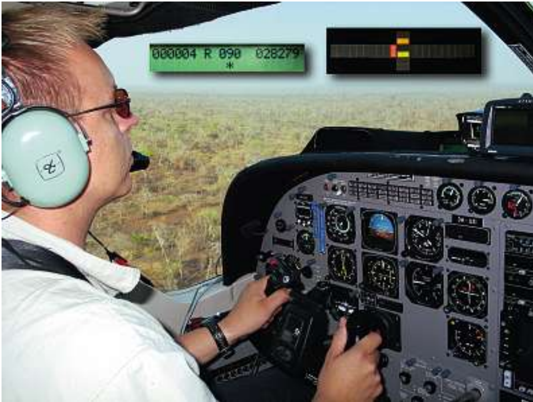
Fig. 28. The LED left-right indicator with green/red colours and numeric display are easily seen when flying along the flight line. Photo: Kai Nyman
