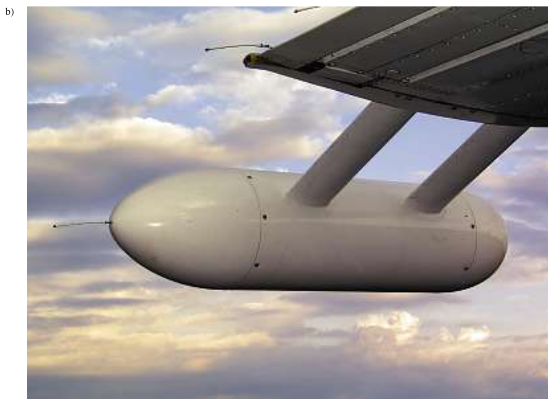
Fig. 7. (a–b). The technique for fitting the EM pod to the wing tip. a) installation and b) the pod. Photo: Kai Nyman
