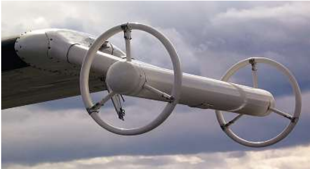
Fig. 6a. The EM wingtip installation in the Twin Otter. Photo: Kai Nyman
