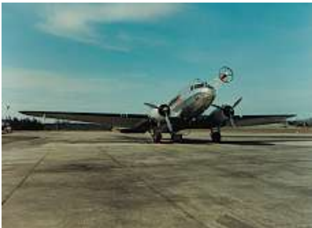
Fig. 6a. Transverse horizontal gradiometer installed at DC-3 (1975–1980 surveys). Photo: GTK archives
