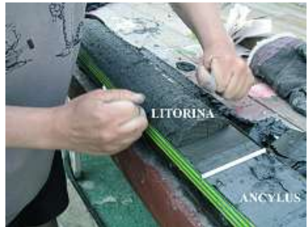
Fig. 18. Splitting the sediment core onboard r/v Geola. White line in Figure indicates the onset of the Litorina Sea stage in lithostratigraphy. (Photo: J. Hämäläinen, 2003).
