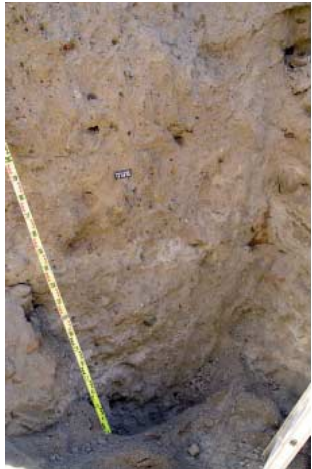
Fig. 3. Two till units in test pit M53 on the proximal part of the drumlin at Korkea-aho, Kuusamo. The upper till unit is composed of homogenous sandy till with fissility, typical of subglacial lodgement till. Lower till includes sorted sandy lenses and bands indicating deposition as subglacial melt-out till. Photo P. Sarala.
