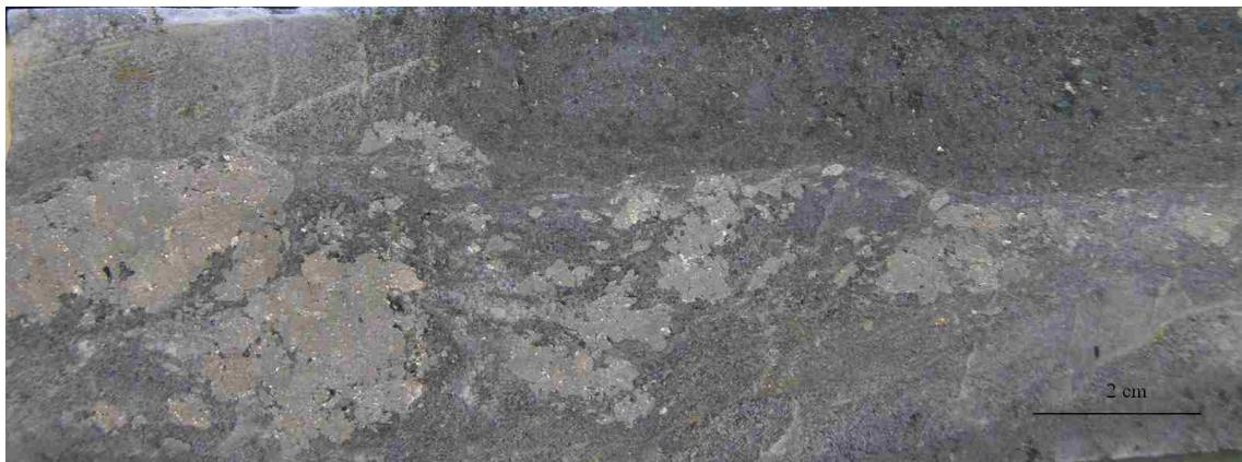
**Quartz, sulphides and gold bearing shear zone in the gabbro. Photo: Saku Vuori:**
