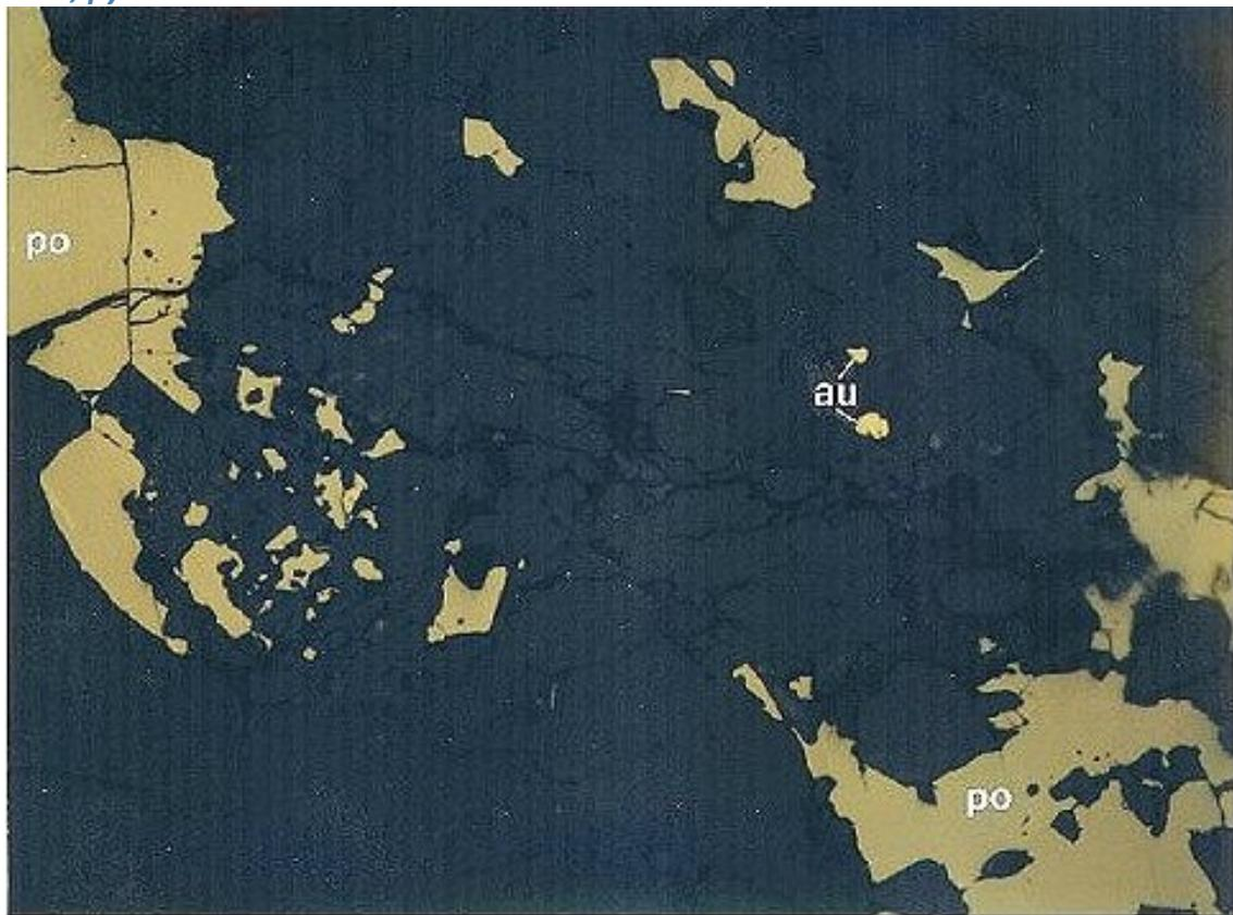
Gold (au) associated with tourmaline in a tourmaline-pyrrhotite (po) aggregate in a quartz vein at Kelokorpi, Ilomantsi. Parallel polarizers, reflected light, field of view 7.5 mm. From Kojonen et al. 1991.
