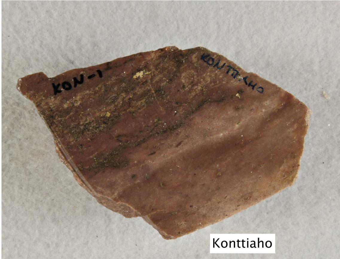
*Sample from the largest pipe. Chiefly quartz-albite-carbonate brecciafill. The host rock fragments probably are intensely altered dolerite with mineral assemblage ab - para - carb*
