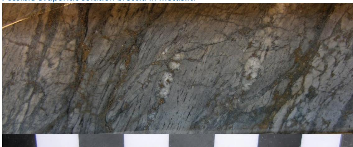
Juomasuo: Possible evaporitic solution breccia in metasilite. Sulphides + albite? + carbonate?
