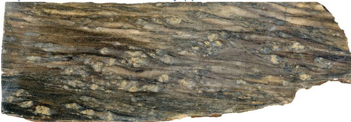
Juomasuo, Kuusamo. Proximal alteration and gold mineralisation in mafic(?) host rock. Mineral assemblage sericite - albite - chlorite - quartz - rutile - pyrrhotite ± biotite. Field of view 15 cm. Photo Jari Väätäinen.
