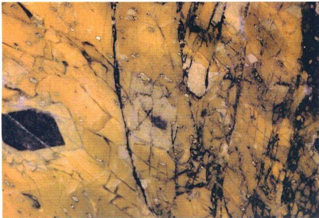
Hangaspuro. Finegrained albite rock with zoned carbonate porphyroblasts and pyrite. Brecciated by later hydrothermal biotite-chlorite filled veins.
