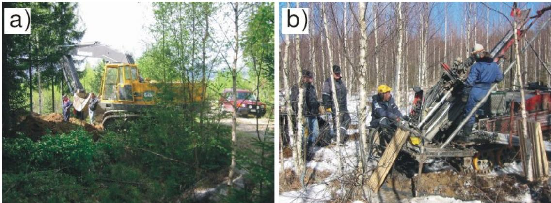
Sampling in the Ritakallio area: a) heavy mineral exploration in till and b) diamond drilling.
