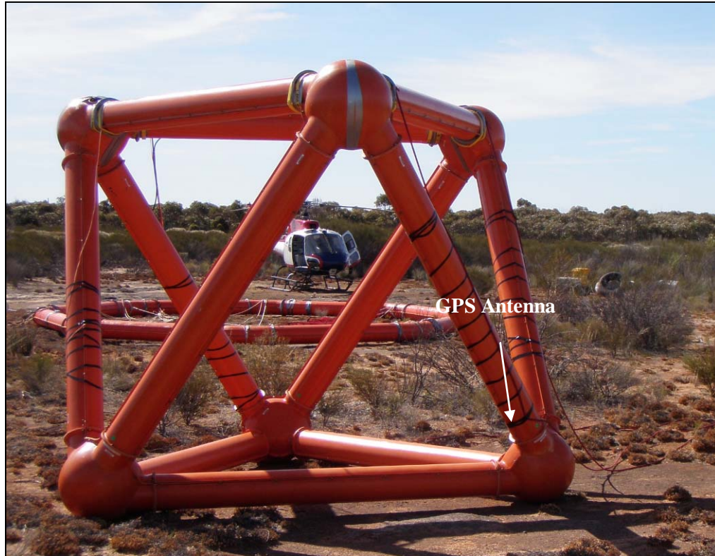
Figure 5: ZTEM base station receiver coils.
