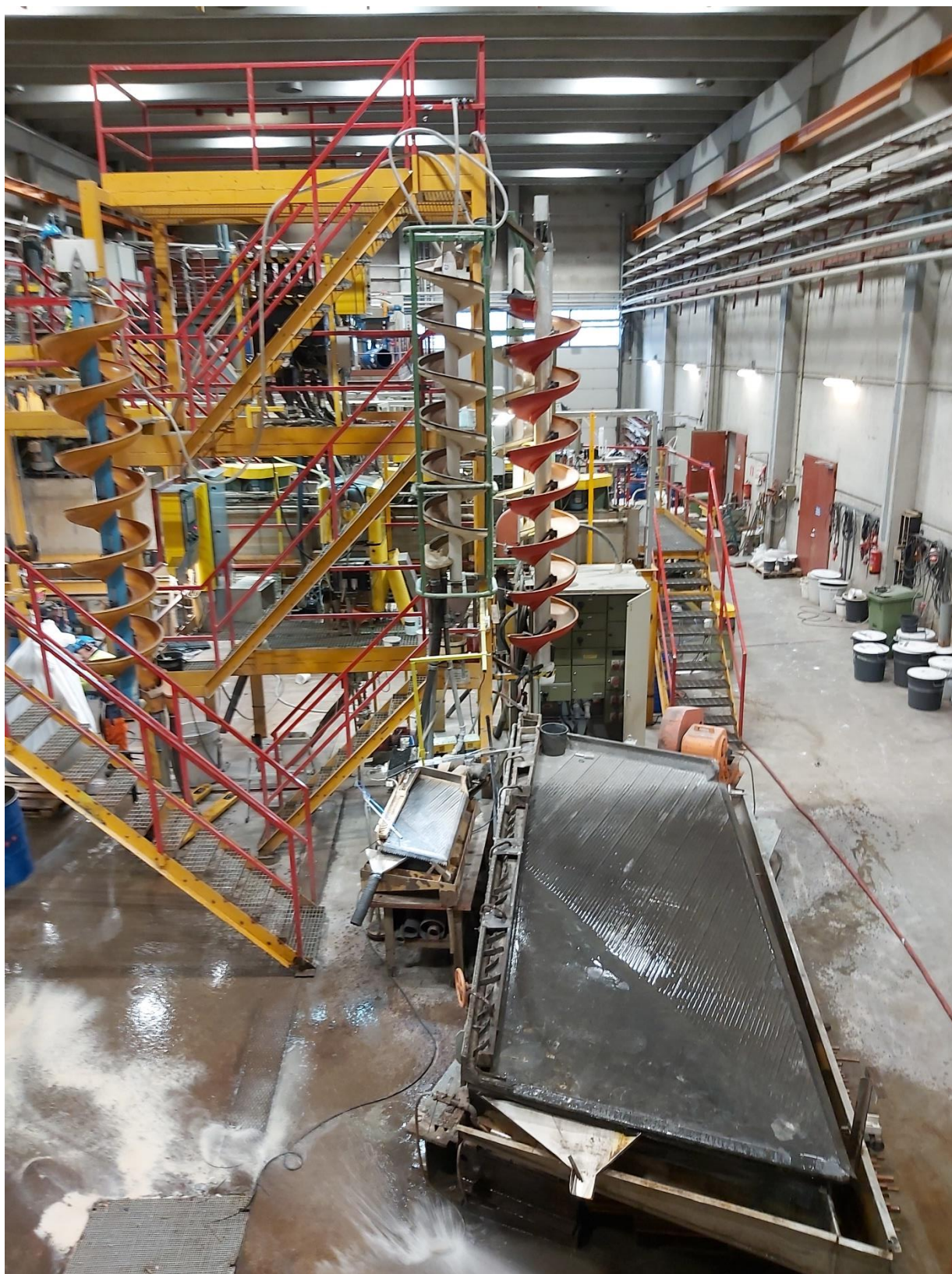
Figure 108. The gravity circuit section of the GTK Mintec process pilot scale plant, gravity spirals and shaking table (Image: Arno-Matti Kirpala)
