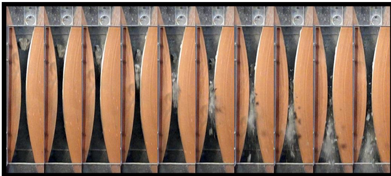
Figure 140. A series of high-speed photographs of a typical crushing event. (Source: Matus et al 2020)
