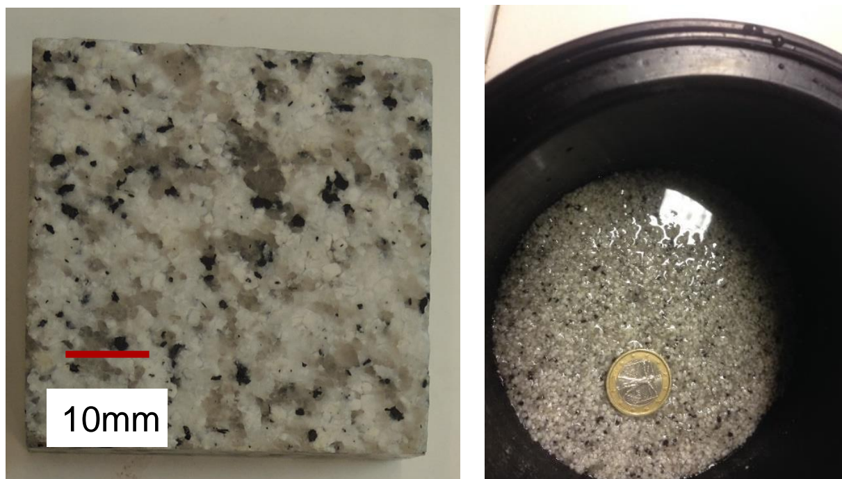
Figure 88. Granodiorite sample intact, before electrodynamic fragmentation (LHS), Same sample just after fragmentation still in the sample holder (RHS) (Michaux 2016) (Image: Simon Michaux)
