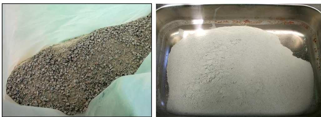
Figure 130. Feed and product samples for the Batch Operating Work Index (Image: Simon Michaux)
