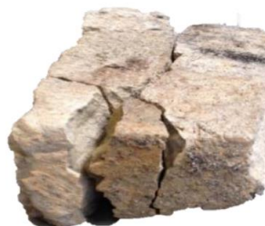
Figure 82. EDF particle body breakage and particle surface breakage
