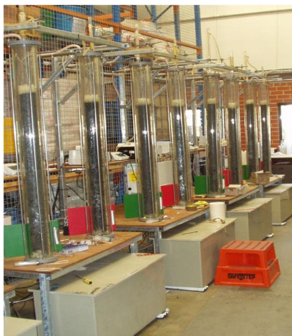
Figure 104. Laboratory scale column leach experimental setup (Source: CSIRO Mineral Resources, Copyright: CSIRO)
