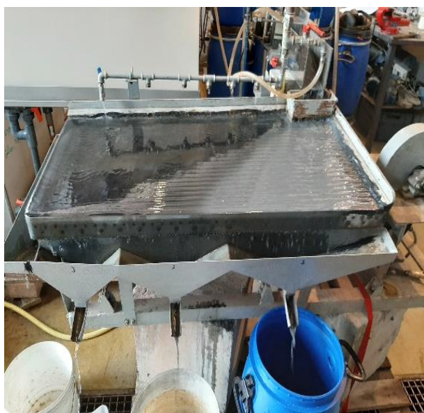
Figure 107. Bench scale shaking table gravity separation (Image: David Bastin & Walter Rivera, ULiege University of Liege)
