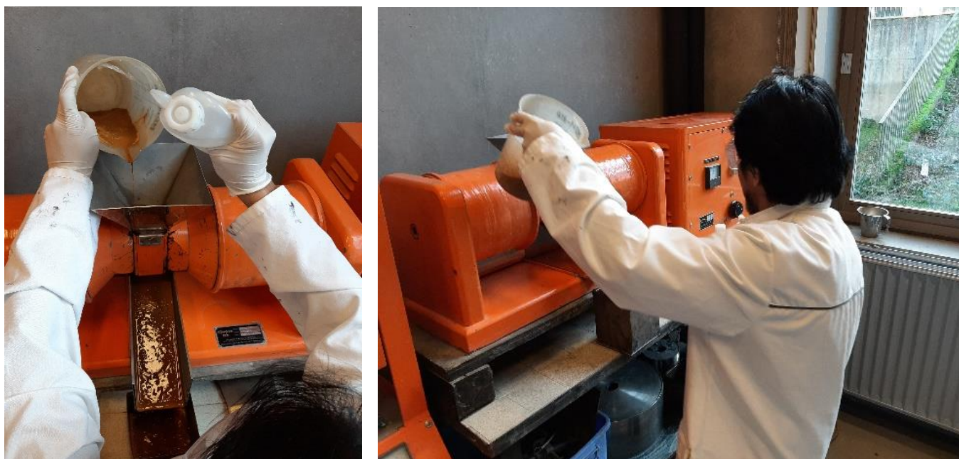
Figure 111. Bench scale magnetic separation process testing (Image: David Bastin & Walter Rivera, ULiege University of Liege)
