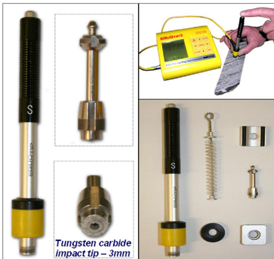
Figure 115. EQUOTip Impact Device (Source: AMIRA P843, AMIRA 2008b, Copyright AMIRA)
