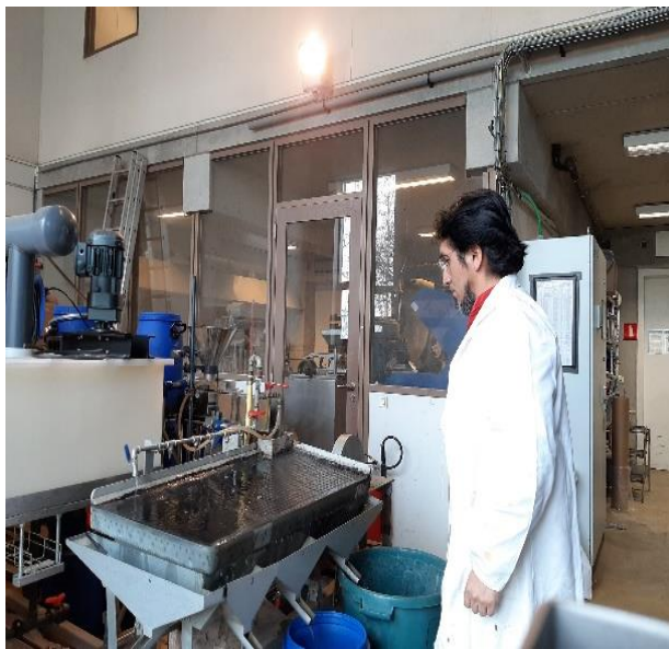
Figure 107. Bench scale shaking table gravity separation (Image: David Bastin & Walter Rivera, ULiege University of Liege)
