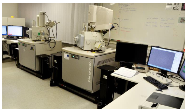
Figure 45. In the foreground is the new FEI Quanta 650 field emission scanning electron microscope, in the background is an older MLA equipment. (Image and copyright: GTK)
