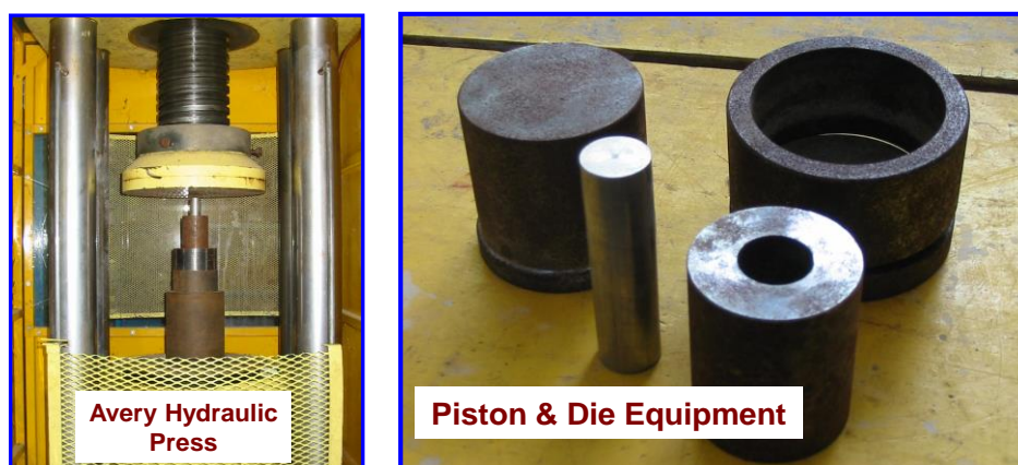
Figure 123. Conventional piston and die unit in a hydraulic press (Image: Steve Walters)
