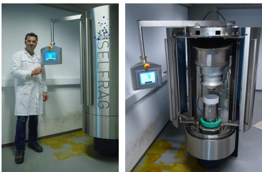
Figure 78. The Selfrag electrodynamic fragmentation instrument (LHS University of Liege ULiege Gemme Dept Unit, Image- Eric Pirard)
