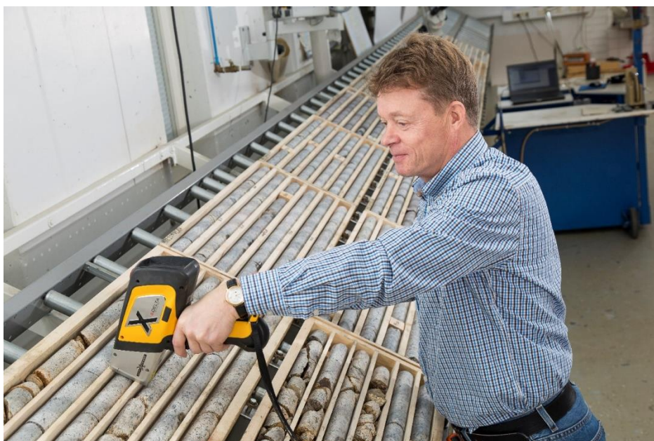
Figure 40. Hand held XRF unit being used on drill core (Image copyright: GTK)
