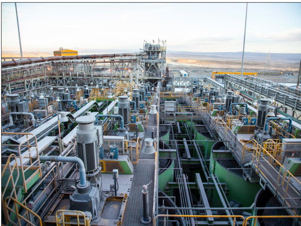
Figure 94. Production scale flotation separation plant (Source: Codelco Flickr, https://www.flickr.com/photos/codelco/ ) (Copyright License: https://www.flickr.com/help/terms )
