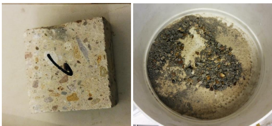
Figure 86. Clean liberation from electrodynamic fragmentation of concrete. The intact 50x50x30mm block (LHS). The fragmented sample after one EDF application (RHS). (Images: Simon Michaux)
