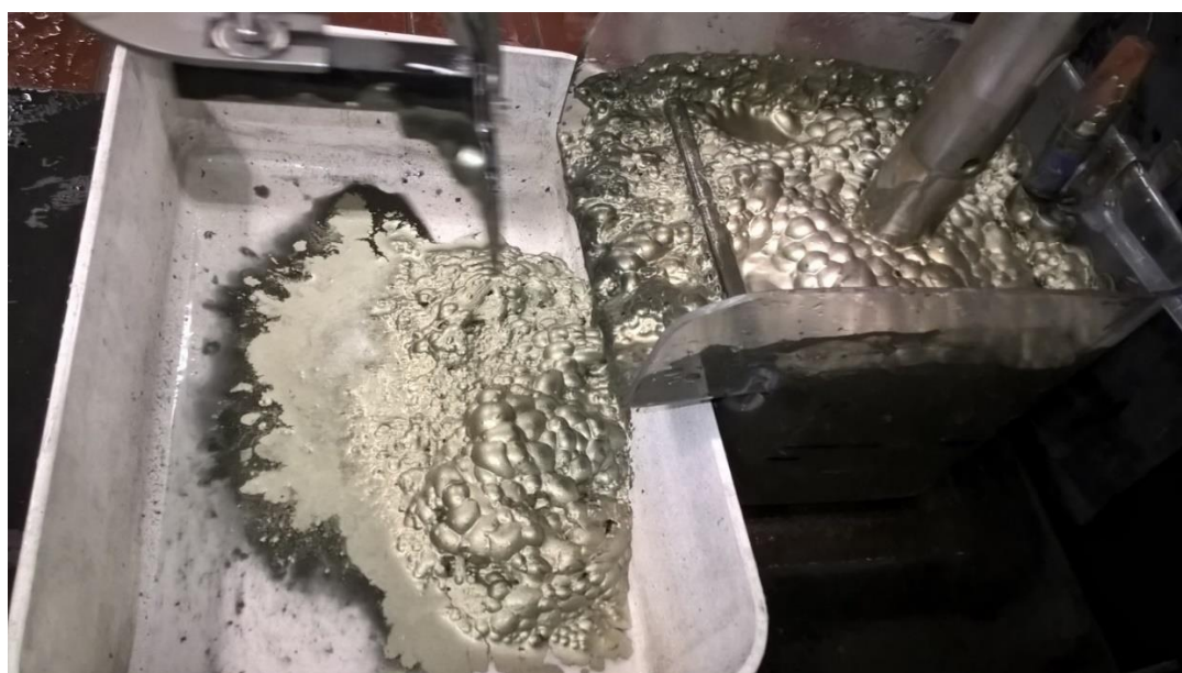
Figure 100. Batch flotation bench scale test (Image: Tero Korhonen)
