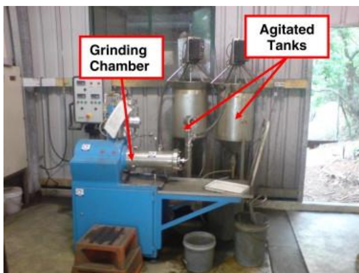
Figure 70. A laboratory scale Isa mill (Image: Simon Michaux)
