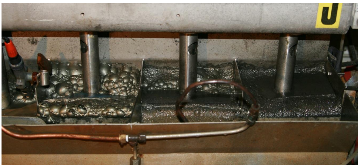
Figure 98. Froth flotation separation (Image: Tero Korhonen)
