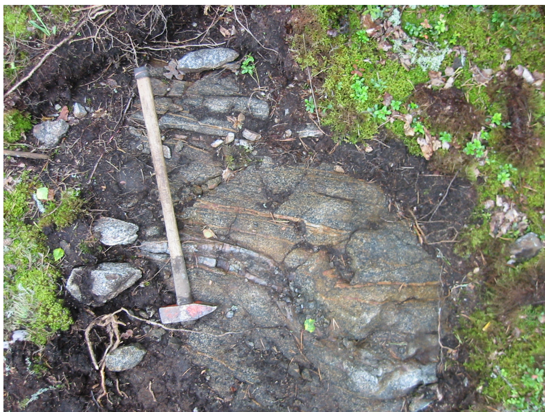
Figure 9. Gold-rich gabbro (1.2 g/t) of Ritakallio typified by quartz veins and shearing (observation 71.4-HML-04). The hammer handle is 60 cm long.
