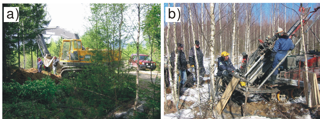
Figure 2. Sampling in the Ritakallio area: a) heavy mineral exploration in till and b) diamond core drilling.
