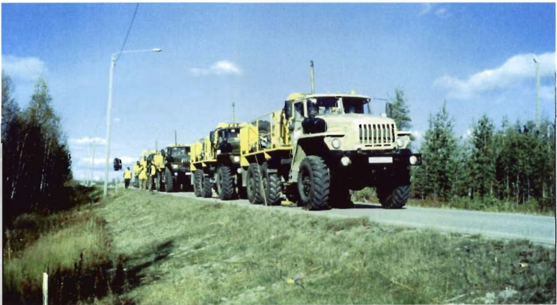
Fig. 1. The vibrator trucks of Spetsgeofizika ready to start the reflection seismic soundings in Vartius, eastern Finland, September 2001. Photo by I. Kukkonen.
