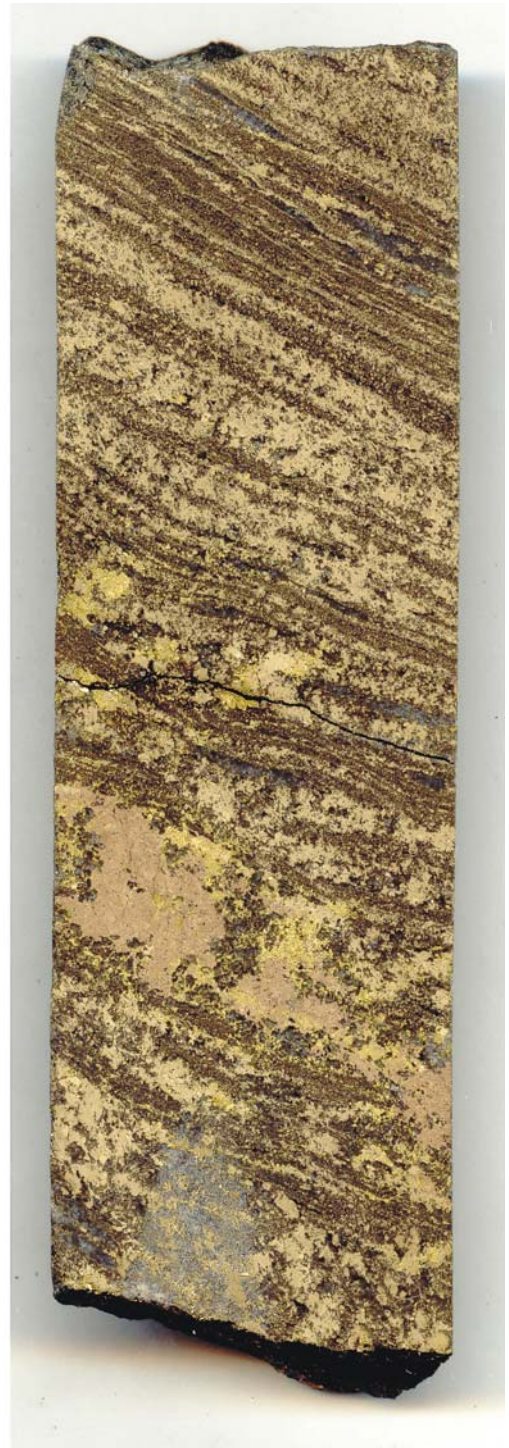
Fig 76. Scanned images of Kylylahti banded byrite ore. The left image shows a fine-grained, more "primary" type with secondary pyrite blebs starting to develop by shearing and associated folding (Oku-902/365.00, height of the slabs ca. 60 mm). The right image shows a more strongly tectonized, banded version probably from a protolith as in the left image (Oku-791B/653.00, width of the slab 30 mm).
