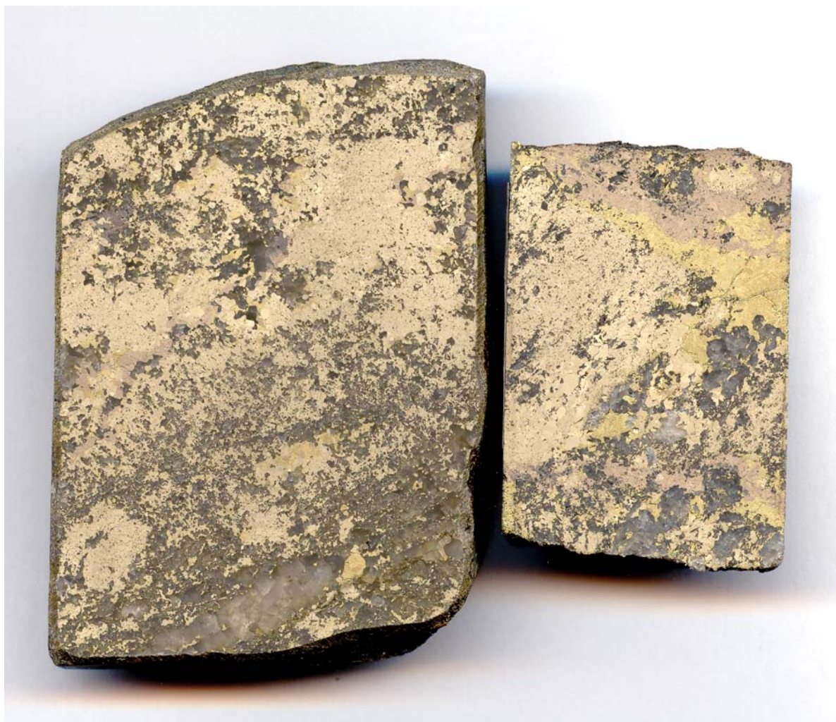
Fig. 54. Scanned images of blebby pyritic ore from Outokumpu (left, Mökkivaara) and Kylälahti (right, Oku-870B/262.60). Note the coarse grain size of the gangue quartz and replacement of the fine-grained pyrite blebs in the both cases by pyrrhotite and chalcopyrite. Width of the samples: left 45 mm, right 30 mm.
