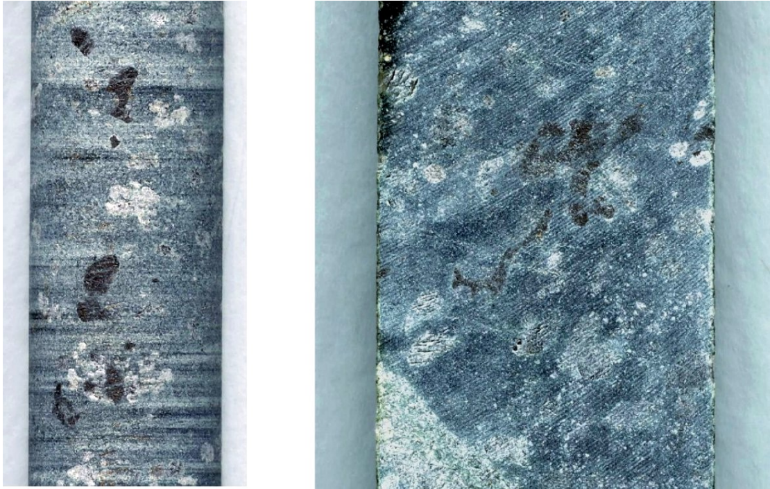
Fig. 16 . Scanned images of two samples of carbonate porphyroblastic antigorite metaserpentinites from southern part of the Kylylahti massif (R393/515.15-515.45). Coarse-grained anhedral, lobate to amoebic chromite grains as in these two samples are typical of the Kylylahti massif and strongly depleted mantle residual peridotites. Similarly coarse grain size and occasionally preserved lobate to amoebic shapes characterize also well-preserved chromite of the other Outokumpu area metaperidotite massifs.
