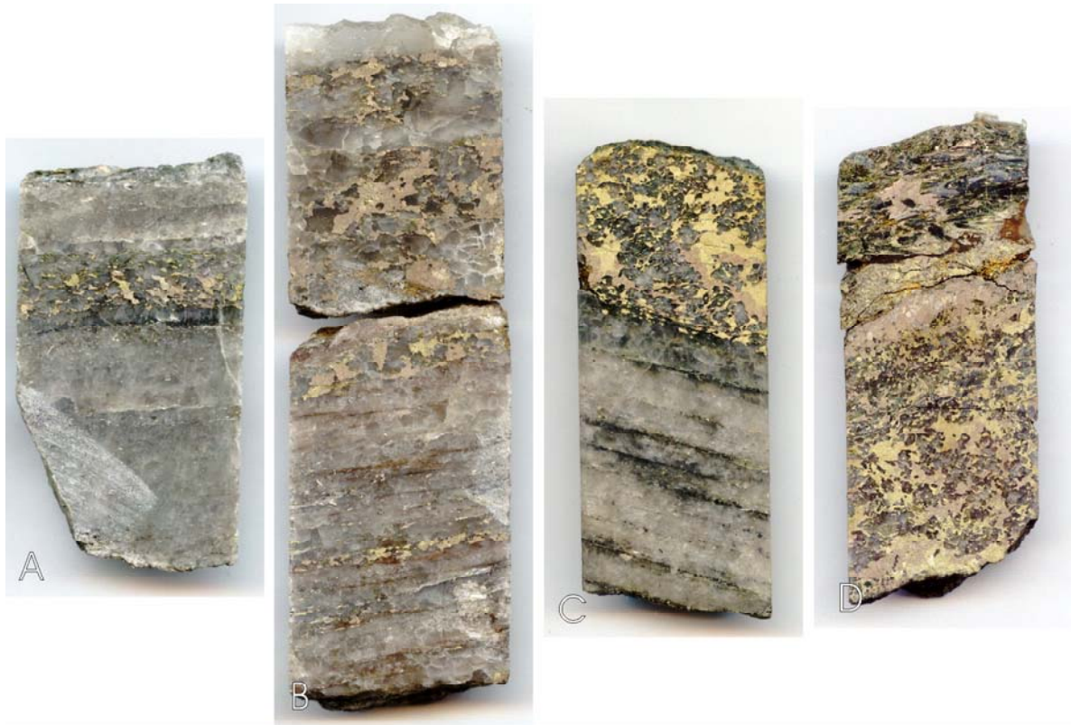
Fig. 57. Scanned images of samples of schistosity-parallel sulphide-quartz bands characteristic of the parallel "Co-Ni zone" of the Outokumpu deposit. (A) Sharply-bound, 12 mm thick chalcopyrite-pyrrhotite-quartz band (vein) in coarse-grained quartz rock, Oku-832/80.82. (B) Chalcopyrite-pyrrhotite-quartz bands in quartz rock, Oku-832/84.10. (C) Very sharp boundary of a chalcopyrite-rich sulphide-quartz band in strongly lineated-schistose quartz rock with cataclastic chromite in thin shear stripes (black), Oku-835/68.40. (D) Sharp boundary of a chalcopyrite-pyrrhotite-quartz band in cordierite-anthophyllite schist (note a seam of massive pentlandite-pyrrhotite between the sulphide-quartz band and the cordierite-anthophyllite schist), Oku-835/72.50. Widths of the half-split drill-core samples are for all ca. 30 mm.
