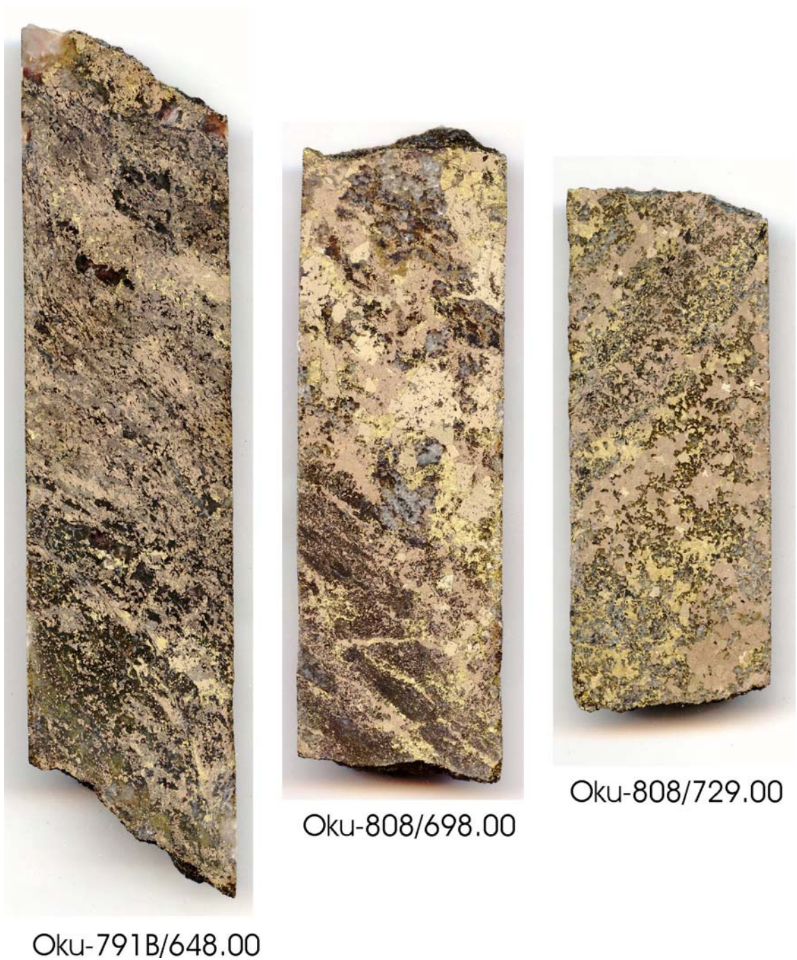
Fig. 78. Scanned images of late metamorphic textures and structures of the Kylylahti massive-semimassive sulphides. (Oku-791B/648.00) Magnetite-pyrrhotite ore from the middle part of the deep ore lens. Note that magnetite and pyrrhotite in this sample enclose schistosity-defining tremolite needles and mica flakes. (Oku-808/698.00) Large retrograde Pyrite IV idiomorphs in pyrrhotite and chalcopyrite that are replacing fine-grained earlier pyrite. (Oku-808/729.00) Chalcopyrite-pyrrhotite ore showing granoblastic intergrowth texture of sulphides and quartz, as it is typical for thoroughly metamorphosed-Outokumpu ores. Width of the slabs 30 mm.
