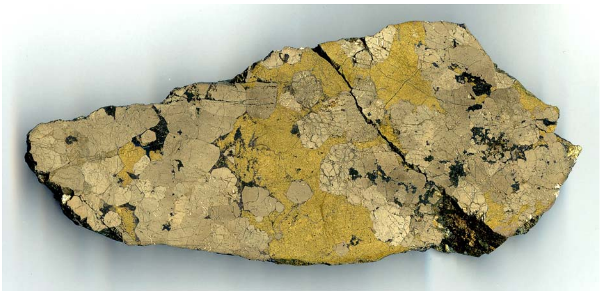
Fig. 102. Scanned image of chalcopyrite-pyrite ore from Luikonlahti, showing large metamorphic Co rich pyrite cubes in massive chalcopyrite. The dark patches interstitial of the sulphides comprise mainly graphite. Width of the slab ca. 12 cm.
