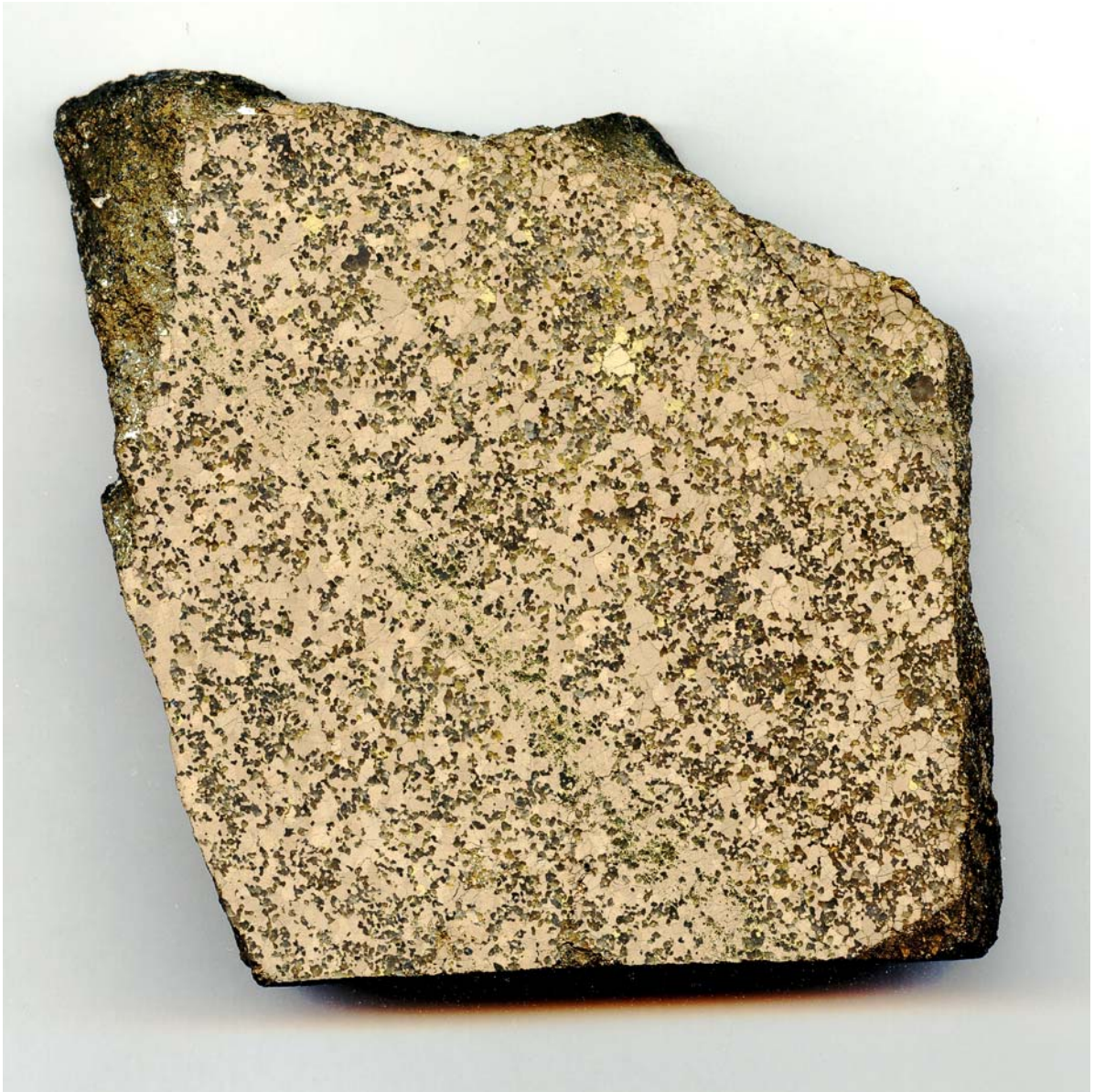
Fig. 101. Scanned image of typical Luikonlahti sphalerite-chalcopyrite-pyrrhotite ore. Note the relatively coarse-grained granoblastic-graphic intergrowth of the sulphides and quartz gangue. Width of the slab ca. 85 mm.
