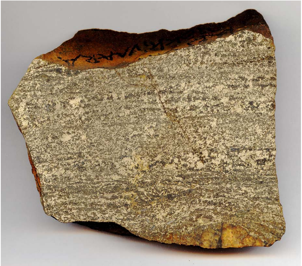
Fig. 53. Scanned image of a sample of blebby-banded pyritic ore typical in the middle parts of the Outokumpu main ore, Mökkivaara, Outokumpu. Width of the slab is ca. 11 cm.
