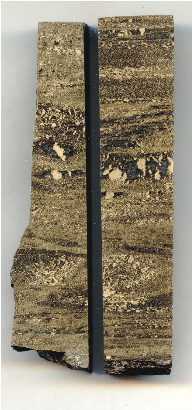
Fig 76. Scanned images of Kylylahti banded byrite ore. The left image shows a fine-grained, more "primary" type with secondary pyrite blebs starting to develop by shearing and associated folding (Oku-902/365.00, height of the slabs ca. 60 mm). The right image shows a more strongly tectonized, banded version probably from a protolith as in the left image (Oku-791B/653.00, width of the slab 30 mm).
