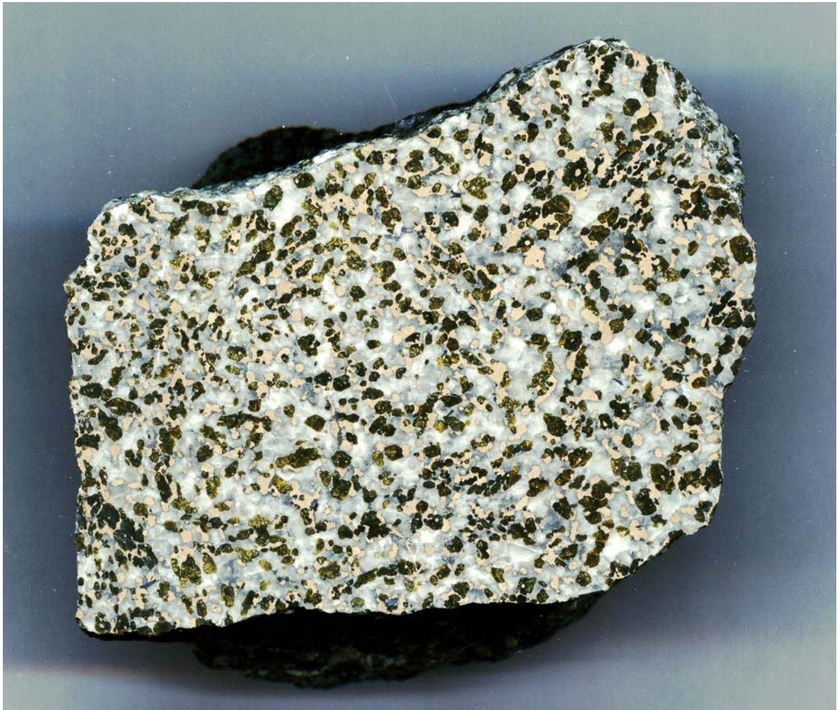
Fig. 97. Scanned image of a sample of pyrrhotite disseminated olivine-carbonate rock typical of the carbonate-skarn zones in the Luikonlahti massif. Dark green=serpentinized olivine, pale grey=carbonate, brown=pyrrhotite.
