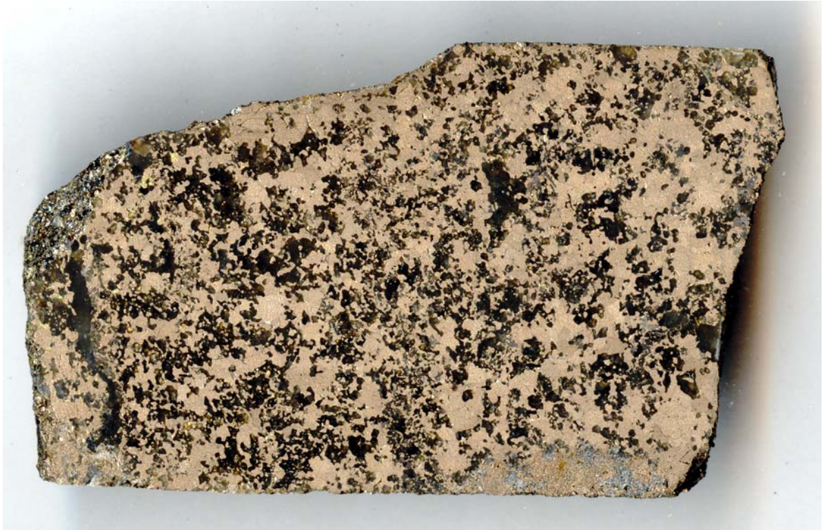
Fig. 112. Scanned image of granoblastic-graphic sulphide-quartz intergrowth texture typical of the Hietajärvi massive ore. Width of the view ca. 70 mm.
