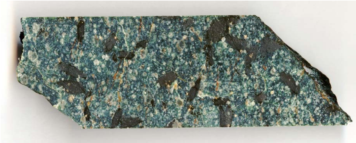
Fig. 17. Scanned image of a sample of olivine-carbonate prophyroblastic antigorite metaserpentinite from the lower levels of the Kylylahti massif (R397/1036.65). Black=olivine, grey=carbonate, green=antigorite.
