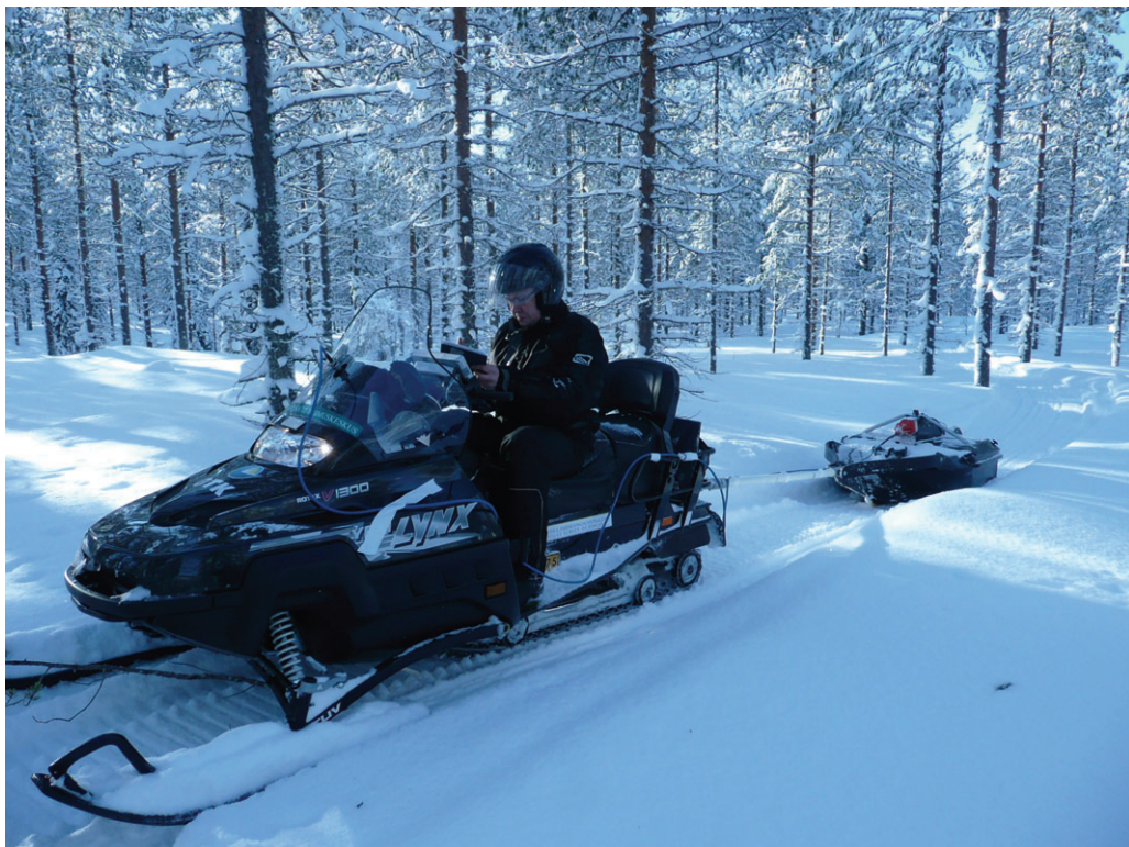
Fig. 1. GPR measurement with snow mobile vehicle. The type of equipment was SIR-3000 with 100 MHz antenna. Photo P. Sarala.
