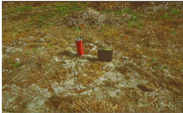
Radioactive crystals of gypsum precipitating in a wetland downstream of a tailings dams – West Rand mining district – South Africa
