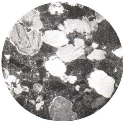
Fig. 10. Secondary growth and corrosion of quartz in the sandstone of Illo in Westanfjärd. + Nicols. Magn. 24 diam.
