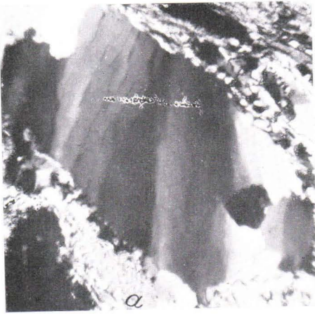
Fig. 8. Relict Böhm striations and ruptural strain shadows. Quartzite from Vaaksaus, Suojärvi. Magn. 20 diam.
