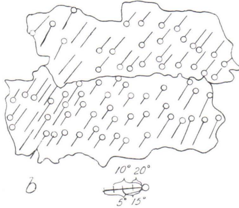
Fig. 9. Quartz grains with Böhm striations from the quartzite of Vittinki. Magn. 25 diam.
