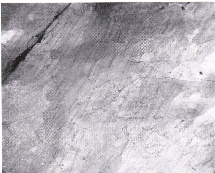
Fig. 10. Böhm striations in the quartzite of Simsjö 4 a. Magn. 30 diam.
