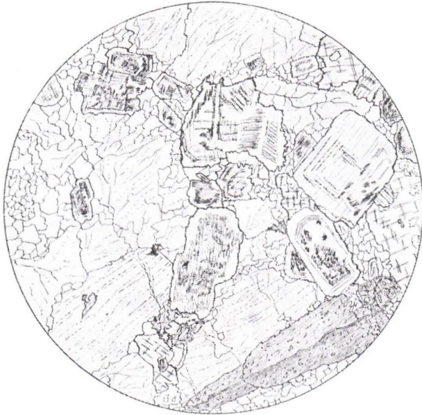
Fig. 16. Slightly granitized granodiorite of Aulanko showing the fine-grained fabric between the primary coarse-grained individuals of granodiorite. National park Aulanko. 7 x.
