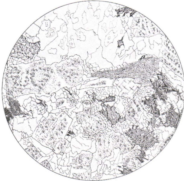
Fig. 22. Epidote-albite rock showing texture relics of the Aulanko granodiorite. Primary plagioclase has altered into epidote and albite. Between bigger plagioclase grains a granitic fabric occurs. The cape at the southern end of Lake Aulangonjärvi. 7 x.
