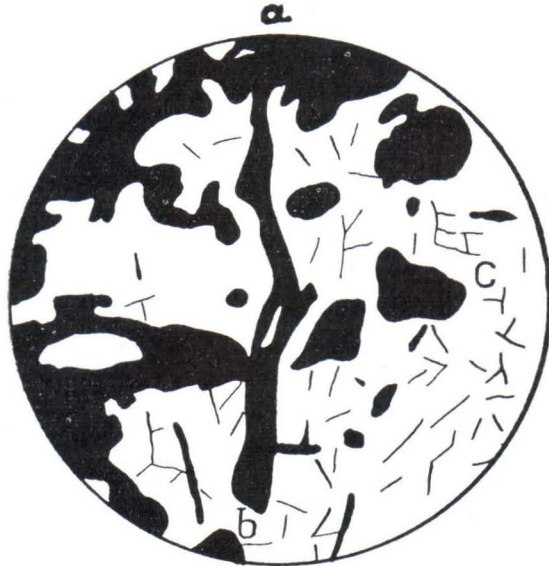
Fig. 6. Wiikite from Lokansaari. White=brownish yellow; black=opaque; a—b and c = lead ore. 100 \times .
