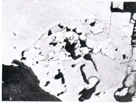
Fig. 3. Gold (light) intergrown with meneghinite (dark grey) in the centre of picture, surrounded by galena (light grey). Black = silicate minerals. Magn. 120 \times .
