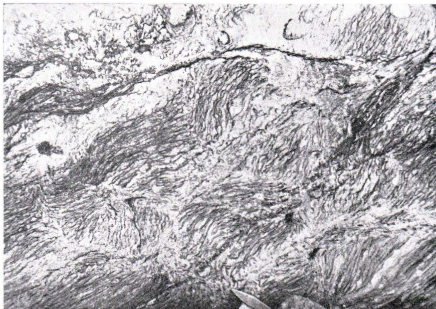
Photo 2. Dictyonite. Elongated metatects of crocydite grown together in a network (compare Sederholm, 1907, pl. IV, 1).
