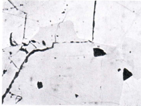
Fig. 4. Meneghinite (slightly darker grey) associated with galena (light grey). Magn. 50 \times .
