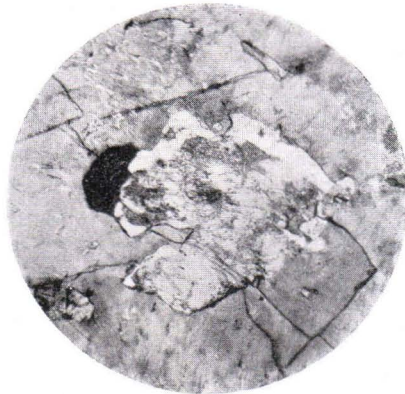
Fig. 39. Shapeless grain of plagioclase with an albitic rim, enclosed by microcline. Microcline granite N. of Lake Paarlahti, Teisko. Nic.+, magn. 40 ×.
