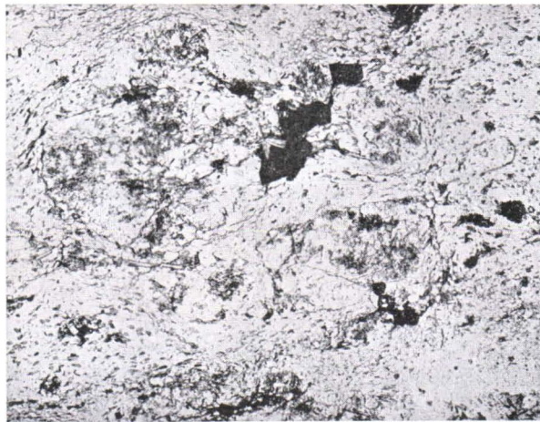
Fig. 45. Silicified schist with pyrite. Turbid spots are plagioclase. W. of Lake Iso Teerijärvi, Orivesi. Nic. ||, magn. 16 ×.
