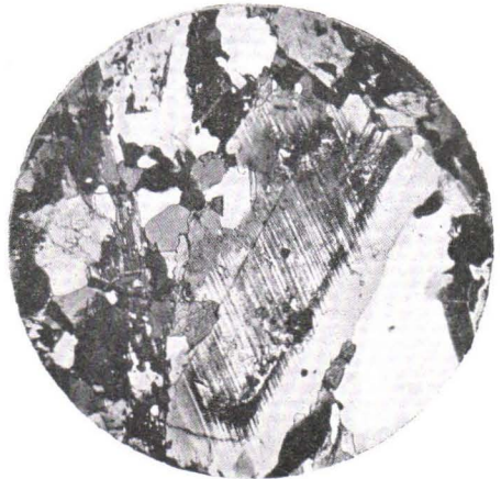
Fig. 26. Plagioclase phenocryst in the schist presented in Fig. 25. Nic.+, magn. 16 | ×.
