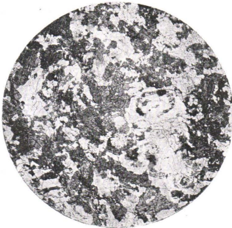
Fig. 28. Recrystallized, gabbro-like variety of basic schist. N. of Lake Paarlahti, Teisko. Nic. ||, magn. 8 \times .
