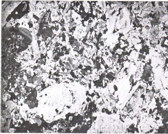
Fig. 25. Plagioclase-porphyritic contact variety of schist. N. of Lake Paarlahti, Teisko. Nic.+, magn. 8 ×.
