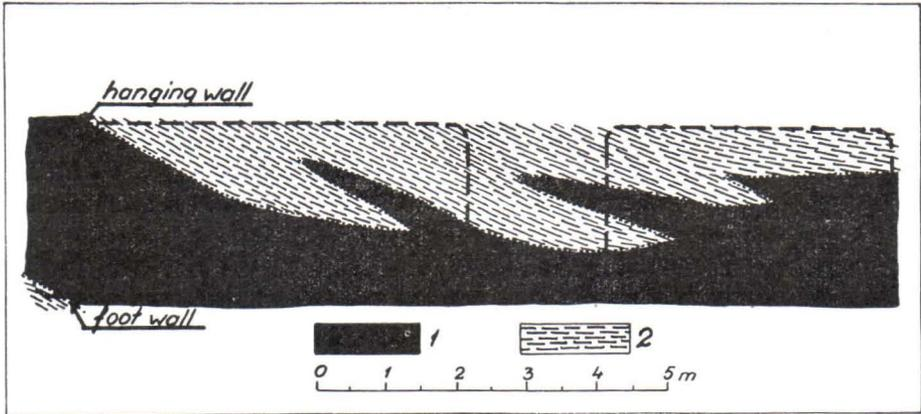
Fig. 8. Intrusion of ore into opened cracks parallel to schistosity in quartzite.
