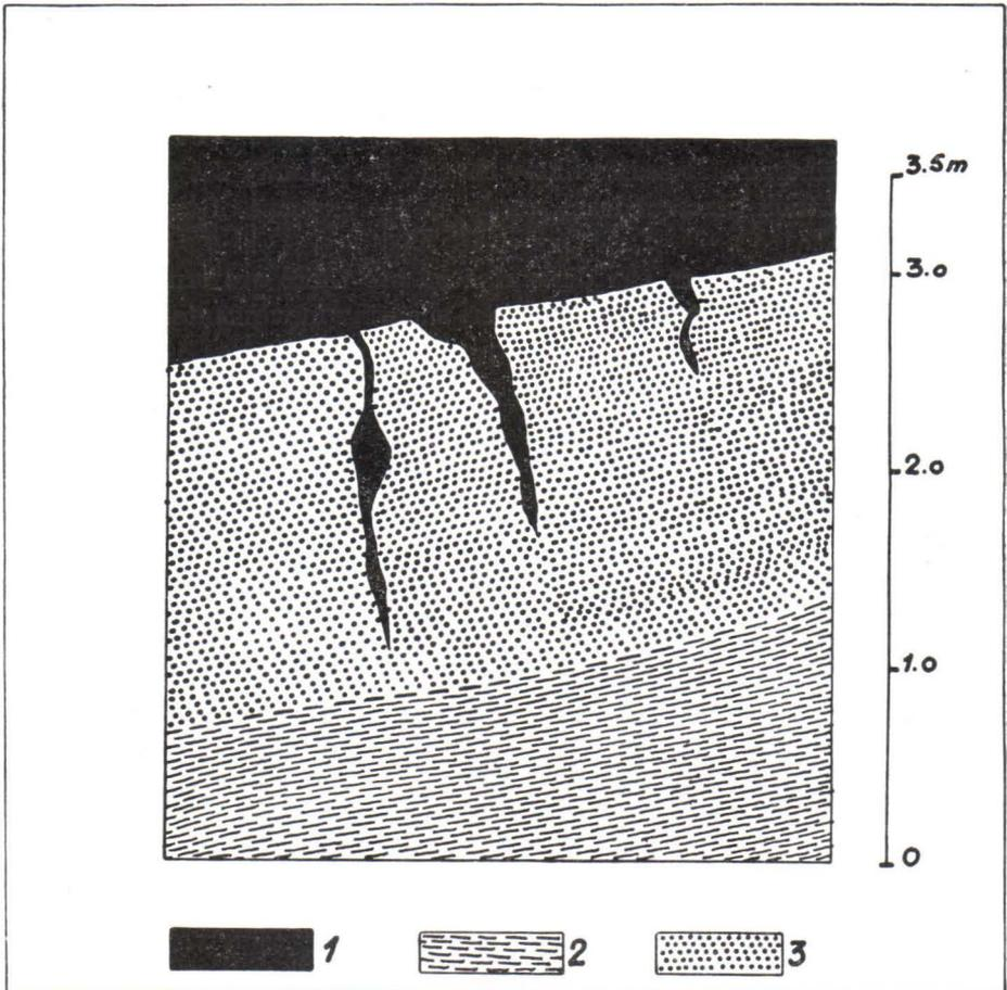
Fig. 9. Ore apophyses in quartzite below footwall. 1. Ore, 2. Quartzite, 3. Quartzite impregnated with pyrite.
