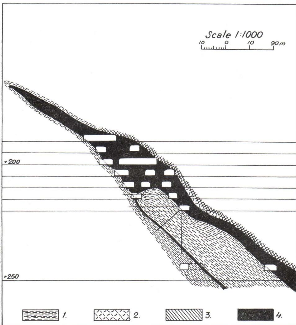
Fig. 7. Cross-section 52—20, showing the displacement of the ore between quartzite layers
