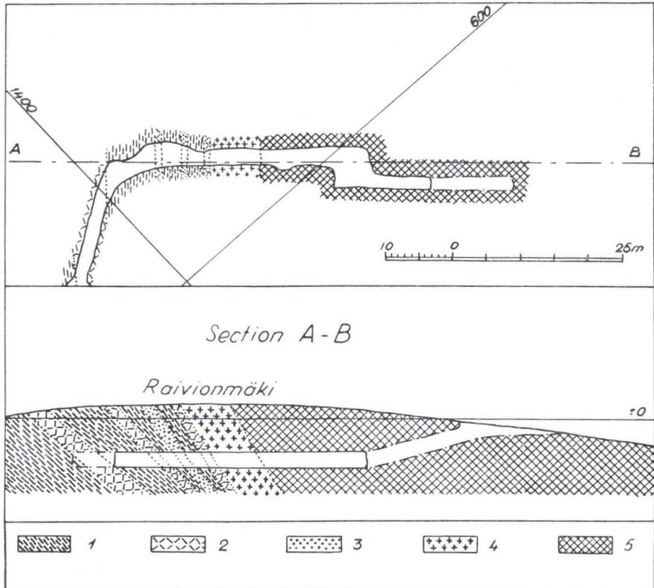
Fig. 4. Prospecting channel at Raivionmäki, Outokumpu. 1. Quartzite, 2. Skarn rock, 3. Anthophyllite-cordierite rock, 4. Dolomite, 5. Serpentine.
