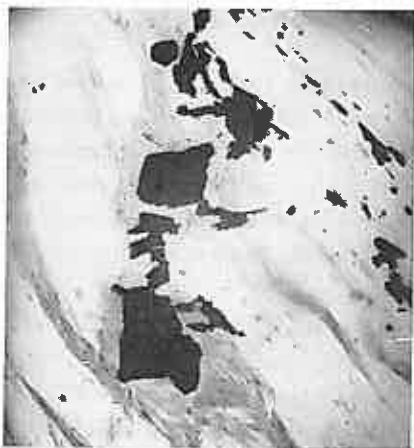
Fig. 7. Soapstone from Handöl, Sweden. Chlorite (grey) arranged around the magnetite grains (black). The main mass of the rock (white) is talc. Mag. 20 \times .
