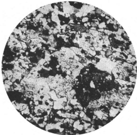
Fig. 2. Poikiloblastic crystal of hornblende (grey) in hornblende schist. A biotite crystal (dark grey) is enclosed by the hornblende. Nic. +. Magn. 50 ×.
