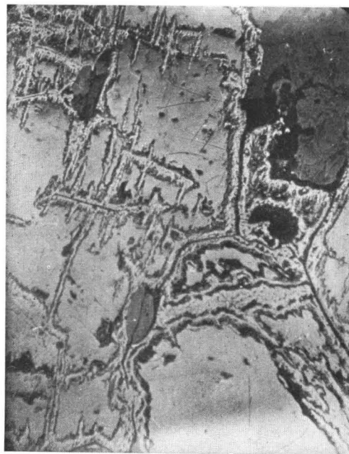
Fig. 8. Marcasite in pyrrhotite. Sulphide-graphite schist. Jalasjärvi. N // x 200.
