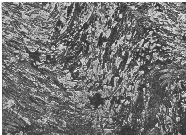
Fig. 6. Sulphide schists of pelitic composition, displaying a miniature-folding, Nokia. N //, 30 \times .
