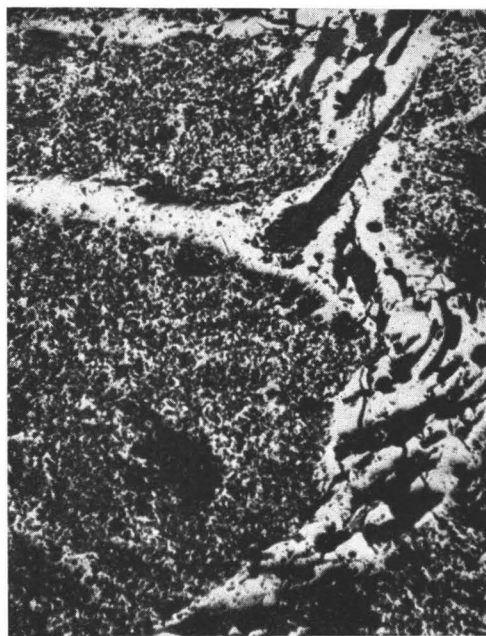
Fig. 4. Two generations of pyrrhotite in the amphibole-sulphide schist of Kaustinen, Österneva. The older generation occurs as a fine impregnation, the younger one as minute veinlets. Pyrrhotite is light. Dark areas are composed of silicates. N //, 40 x.
