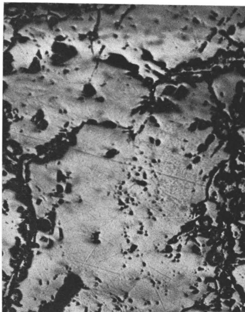
Fig. 2. Pyrrhotite of an amphibole-sulphide schist of Evijärvi. In the pyrrhotite there are narrow cracks filled by concentrically grown pyrite and marcasite. N //, 40 x. See the next Figure.
