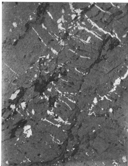
Fig. 7. Pyrrhotite occurs in the cracks of pyroxene. Nokia. N // x 60.
