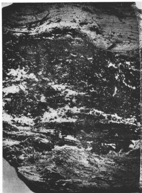
Fig. 5. Three generations of pyrrhotite in the sulphide schist of Kaustinen, Tastula. The oldest generation: thin dissemination; the second generation: gray strips near the edges of figure, consisting of dull pyrrhotite, third generation: bright patches in the center of figure. Ordinary light. 2 x.
