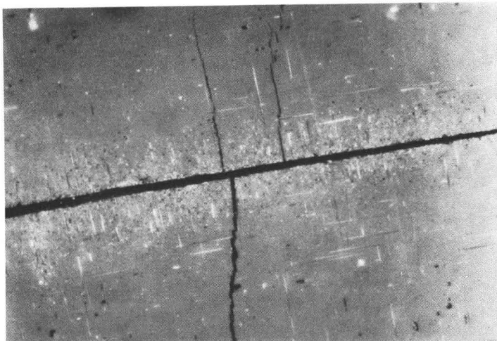
Fig. 1. Alteration spots and lamellae pattern along the crack borders in the chromite. x 650, oil.
