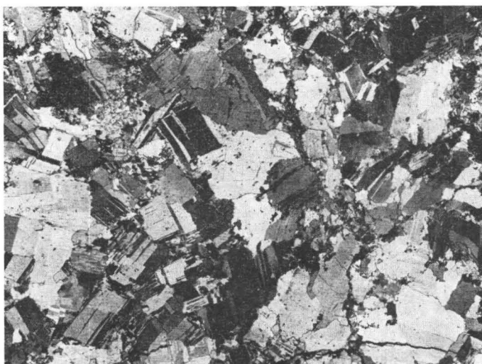
Fig. 15. Hypidiomorphic texture of medium-grained albitite. Iso-Kurkkio, Enontekiö, Finland. Nicols crossed. Magn. 11 \times . Photo E. Halme.
