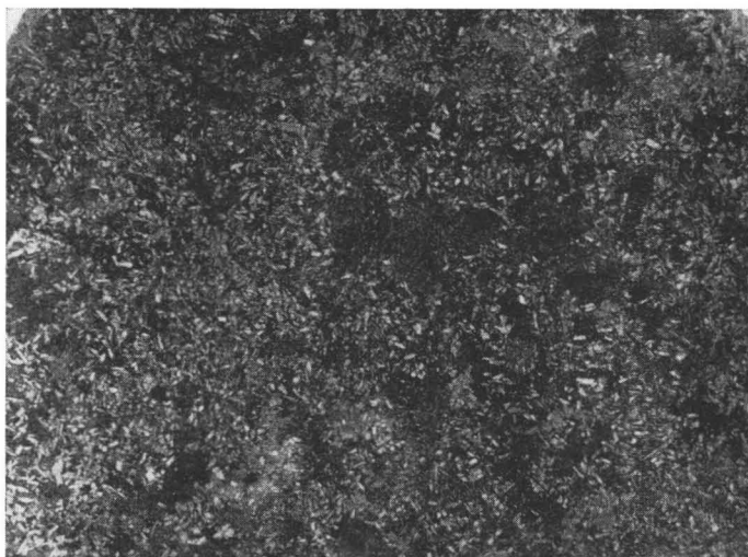
Fig. 6. Glomeroporphyritic and ophitic structure of amphibole-albite rock. Glomeroporphyritic aggregates are composed of hornblende and biotite. Nat. size. Hukkakumpu, Kittilä. Photo E. Halme.
