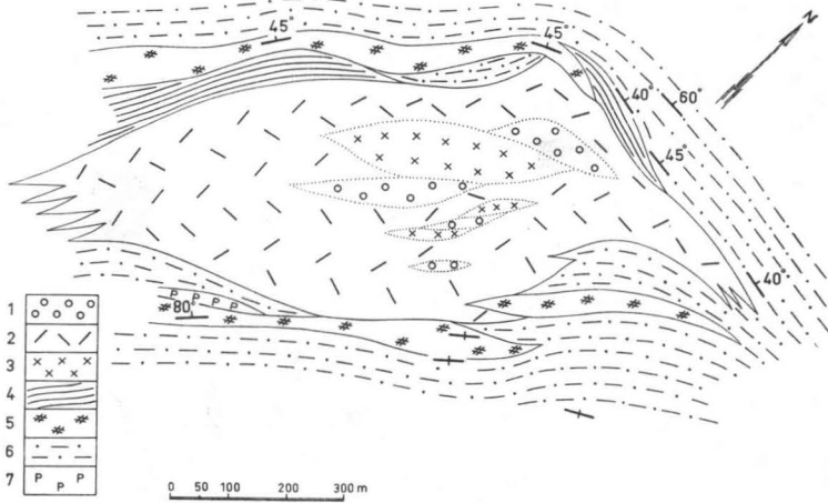
Fig. 14. Molybdenite-bearing latekinematic granite in the crest of a gentle fold. Wankatane River, Sierra Leone. 1 = porphyroblastic granodiorite; 2 = latekinematic aplitic granite; 3 = latekinematic granite containing \text{MoS}_2 ; 4 = fine-grained gneiss; 5 = amphibolite; 6 = schist rich in talc and serpentine; 7 = pegmatite.
