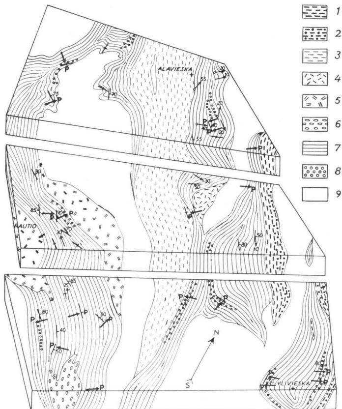
Fig. 7. The structure of the Alavieska, Rautio and Ylivieska schist zones. 1. Amphibolite, 2. Porphyritic amphibolite, 3. Quartz-feldspar schist, 4. Plagioclase porphyrite, 5. Coarse ophitic plagioclase porphyrite, 6. Agglomerate schist, 7. Graywacke-like schist, 8. Conglomerate, 9. Plutonic rocks. P. Direction of the base of the beds.
