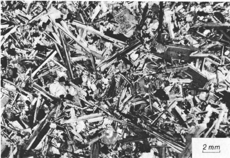
Fig. 2. Ophitic texture of olivine diabase from Ansio. (Microphoto. Thin section, + nic.) Padasjoki, Finland.
