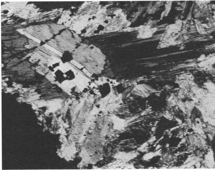
Fig. 6. Stearitized chlorite embedded in hornblende lamina. Amphibole-bearing talc schist. Ahola (29), Sonkajärvi. Nic +, 81 x.
