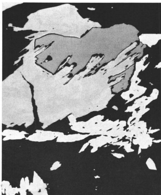
FIG. 46. Dark grey pyrrhotite is partly replaced by medium grey berthierite. White is gudmundite. Polished section. Syrjämo. Drill hole no. 3 (150.35 m). One nicol. Magn. 150 x. Photo E. Halme.
