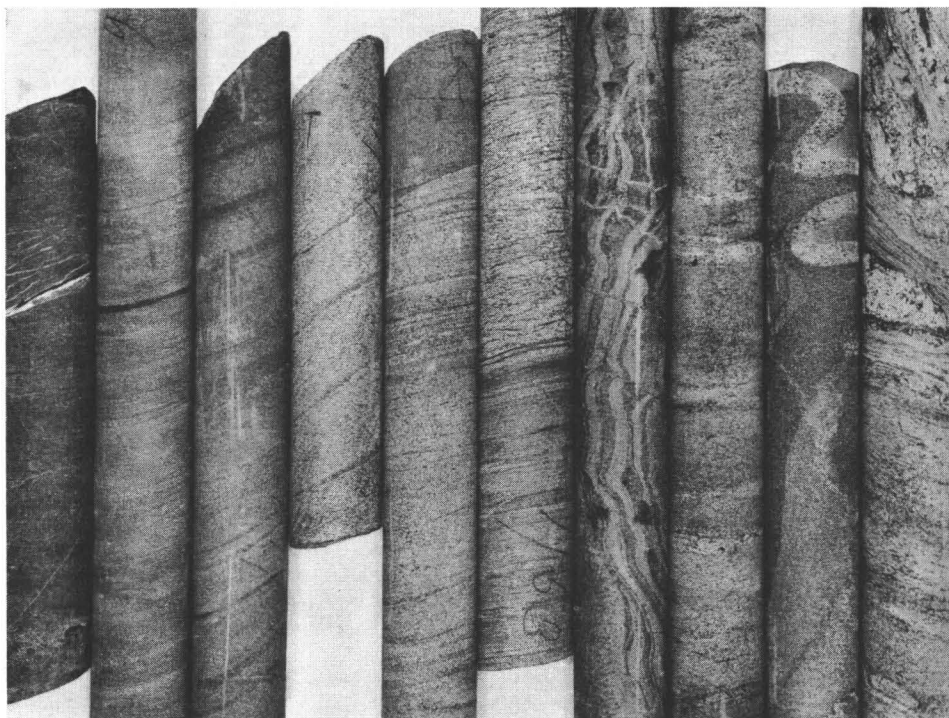
FIG. 32. The different schist types in the Törnävä ore field. Half of the natural size. Photo E. Halme. 1. Graphite phyllite with white calcite as fissure veins. 2. Phyllitic mica schist. 3. Phyllitic schist with varying lamination. 4. Laminated mica schist. 5. and 6. Mica schist and gneiss alternate. 7. Laminated and folded mica schist. 8. Phyllite, rich in quartz. 9. Folded phyllite, rich in quartz. 10. White pegmatite veins in mica gneiss.
