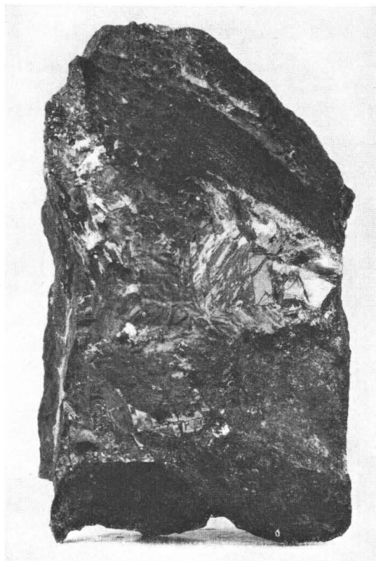
FIG. 2. Specimen of Malinen's boulder. Light grey is native antimony and dark grey is chiefly quartz. About half of the natural size. Photo E. Halme.
