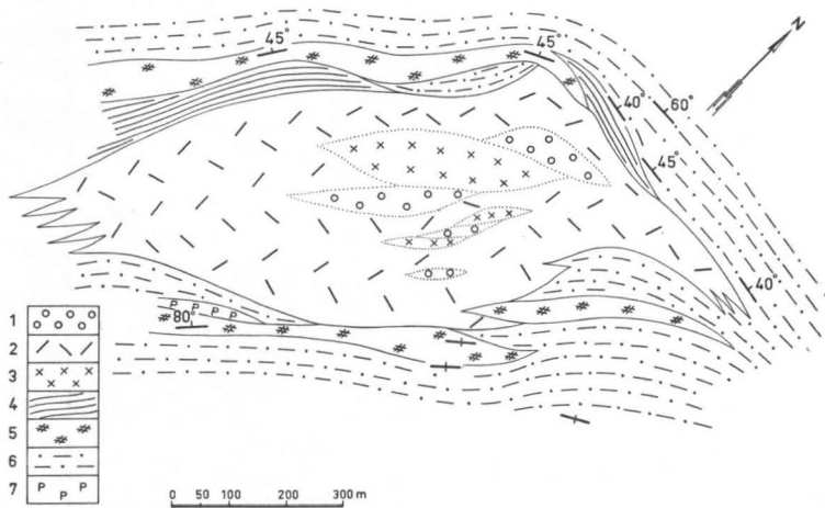
FIG. 17. Molybdenite-bearing latekinematic granite in the crest of a gentle fold. Wankatane River, Sierra Leone. 1 = porphyroblastic granodiorite; 2 = latekinematic aplitic granite; 3 = latekinematic granite containing MoS 2 ; 4 = fine-grained gneiss; 5 = amphibolite; 6 = schist rich in talc and serpentine; 7 = pegmatite
