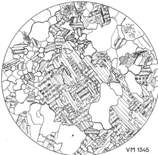
FIG. 23. Microcline replacing plagioclase in a synkinematic granite. At the upper end of the latter there is younger and perfectly fresh albite. South of the Kangari Hills, Sierra Leone. Magn. 40 x.
