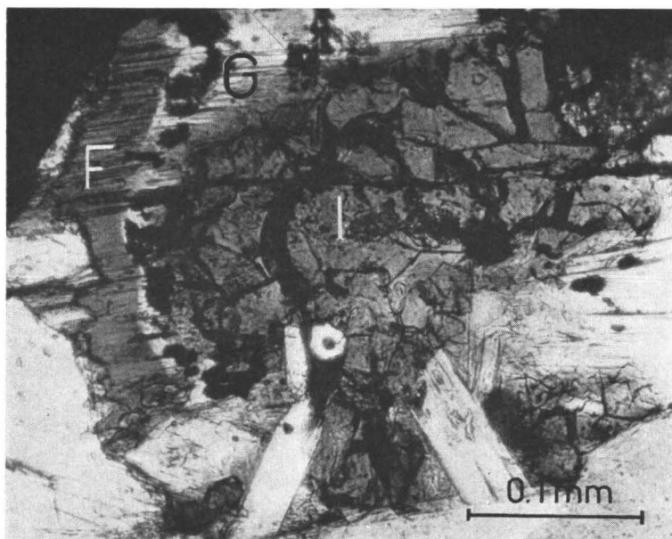
FIG. 3. Grunerite rim ( G ) between ferrohastingsite ( F ) and iddingsite ( I ). Dark-coloured wiborgite (785/ML/54). Tutka-asema, Valkeala.
