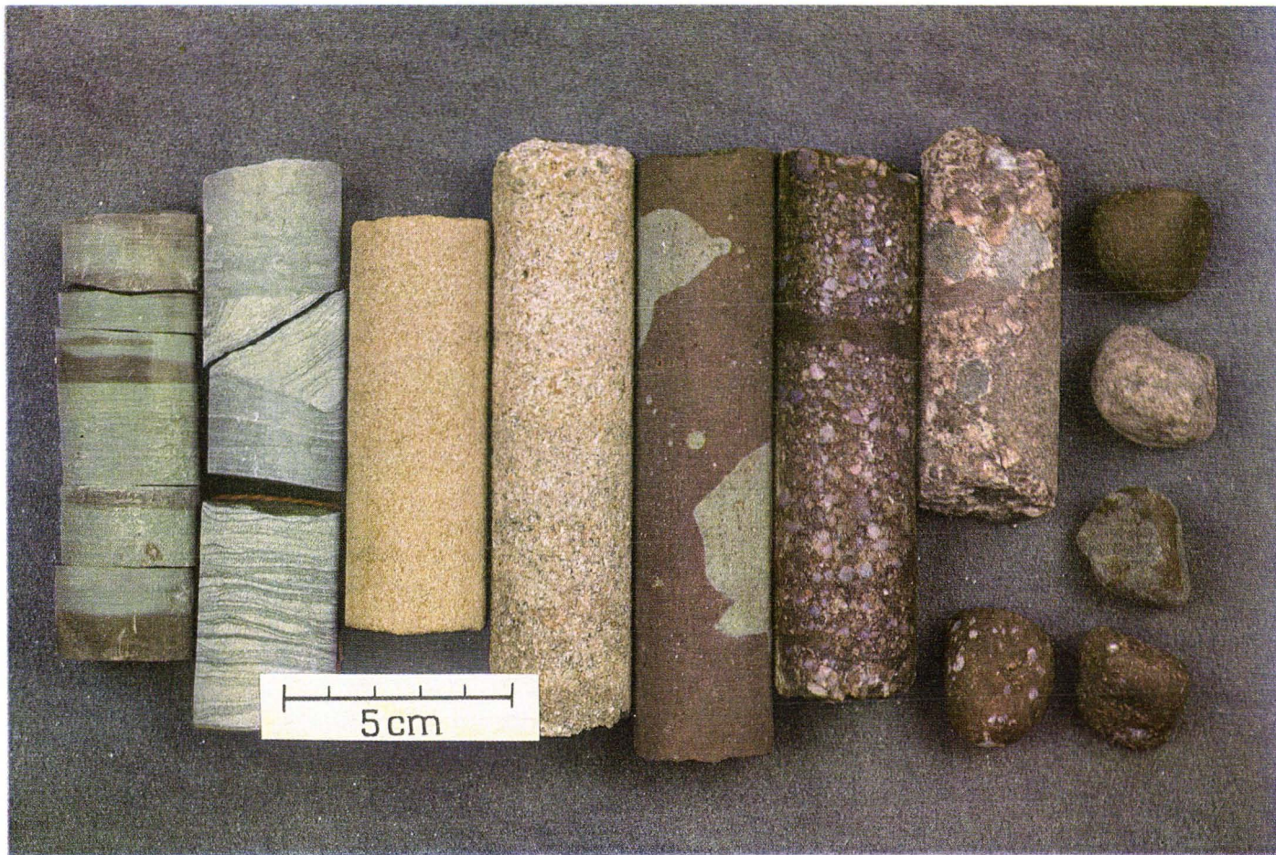
FIG. 11. Typical rock samples from the sedimentary succession in Hailuoto. From the left: shale, siltstone (mixed with shaly matter), sandstone, arkose, red-shale (showing green shale spots), red-arkose (showing red-shale interlayer), conglomerate, rock pebbles detached from the conglomerate. Photo E. Halme.
