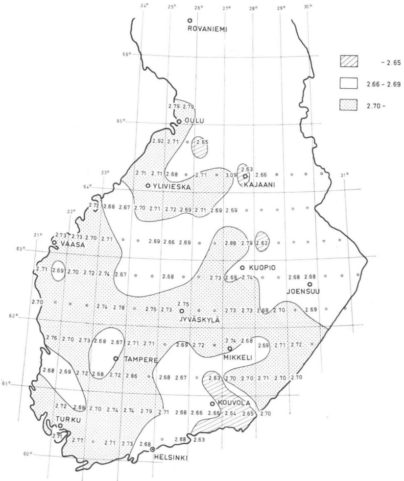
FIG. 19. Geographical distribution of specific gravity of bedrock material.
