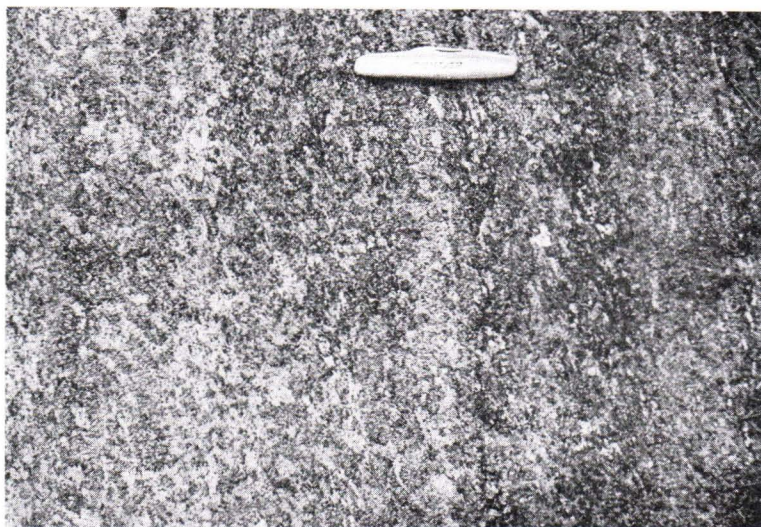
FIG. 8. Banded structure in the metasomatically altered rock. The dark portions are more or less chloritized porphyroblasts of cordierite. Sukulanrakka hills, Hirvas, Rovaniemi. 1/3 natural size.
