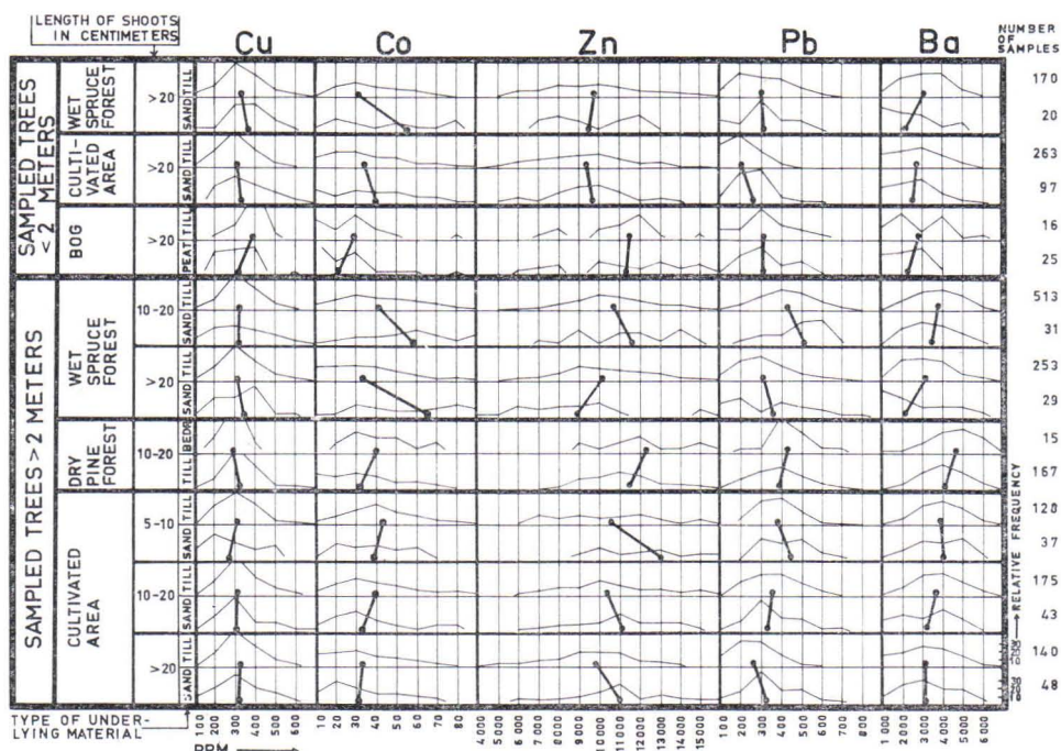
FIG. 9. Medians (filled circles) and frequency polygons of copper, cobalt, zinc, lead and barium contents in the ash of birch twigs sampled above different types of material.
