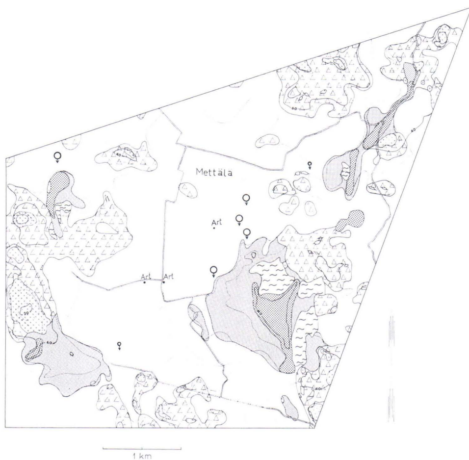
FIG. 12. Typical level clay tract. Ground water formed on glaciofluvial deposits is discharged from sand and gravel layers underlying clay beds as springs as well as from artesian dug wells. Mettälä, Elimäki.
