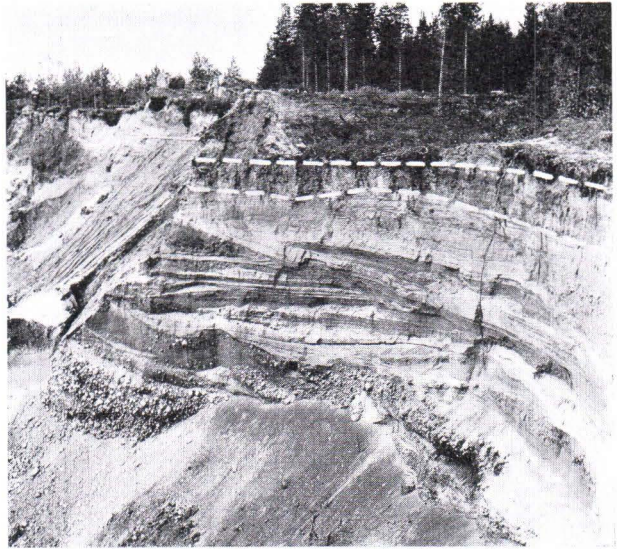
FIG. 3. Section through a broad, level esker. Layer indicated by broken line consists of clay, which is overlain by shore deposits. Interior of esker consists of stony material. Siltakylä, Pyhtää.
