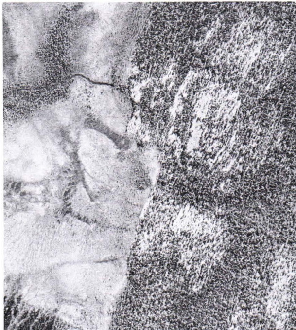
FIG. 33. A slope of a hill covered by block fields and a thin till sheet. Ground water discharges into the bog through a large spring and a seeping belt. In the aerial photograph the block field can be distinguished from the more forested till deposits by its lighter shades. The smoothed tectonic traces of the weathered bedrock, which are probably the bedding of quartzite (cf. heavy lines in Fig. 34), are distinctly visible in the aerial photograph. In the southwestern corner there are light peat ridges in wet bog. The latter shows up as dark patches. By courtesy of Topografikunta (The Army Map Service).
