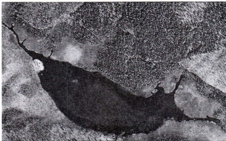
FIG. 30. Ground water discharges into Lake Suasjärvi through the inlets penetrating the alluvial bog and the springs at the foot of the hill. By courtesy of Maanmittaushallitus (The National Board of Survey).
