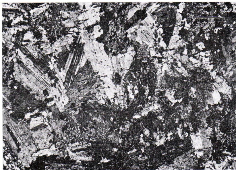
FIG. 37. Ophitic textural features in gabbro. Brändholm, Pernaja. Microphotograph, magnification c. 12 \times , nicols+. Photo Erkki Halme.
