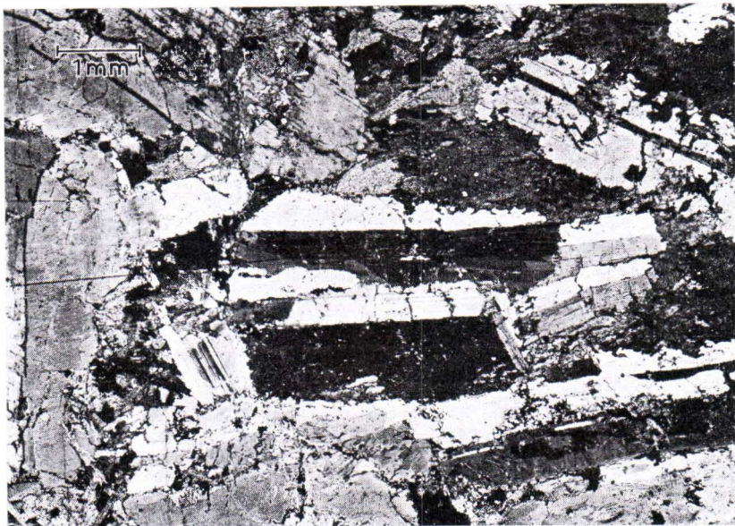
FIG. 39. Gabbro. Strömmingsgrund, rural commune of Porvoo. Microphotograph, magnification c. 13\times , nicols \perp . Photo Erkki Halme.
