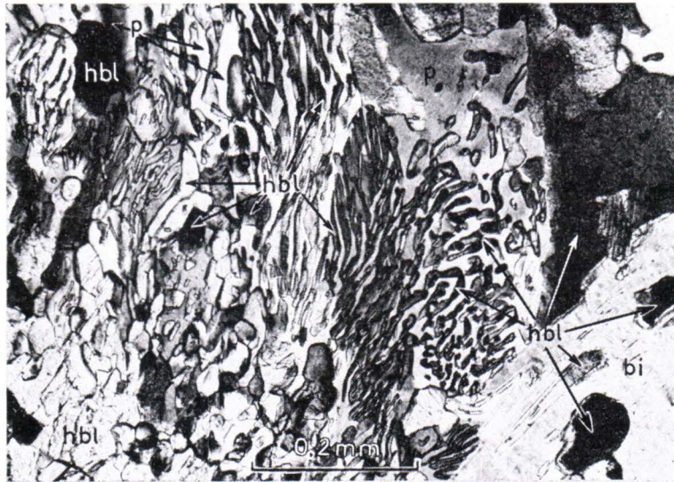
FIG. 15. Hornblende-plagioclase myrmekite. p, plagioclase; hbl, hornblende; bi, biotite. Gabbronorite, sample No. 231a/KV/65. Crossed nicols.
