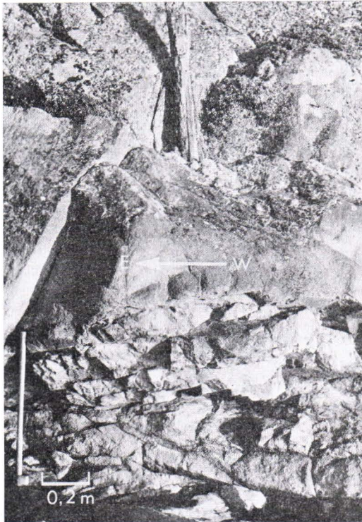
FIG. 10. A crush zone in gabbro with joints, shear fractures and mylonitic portions, and dipping gently south.
