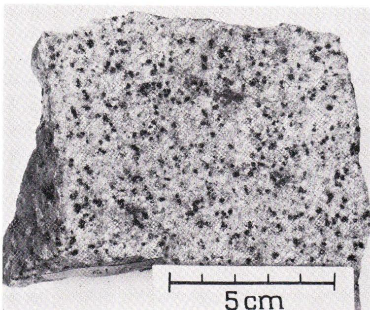
Fig. 19. Fine-grained spotted granite. Sampling site No. 29 in Plate 1. Kodisjoki. Photo: Erkki Halme.
