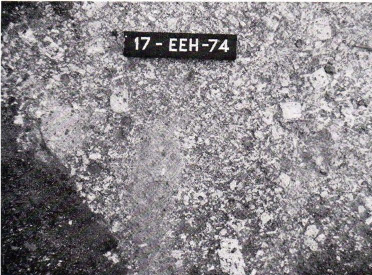
Fig. 28. Fine-grained aplitic autoliths with alkali feldspar phenocrysts in Suutila granite. Southeastern part of the Suutila—Katinhätä complex. Near sampling site No. 39 in Plate 1. Suutila, Karjala. 1/4.0 natural size.
