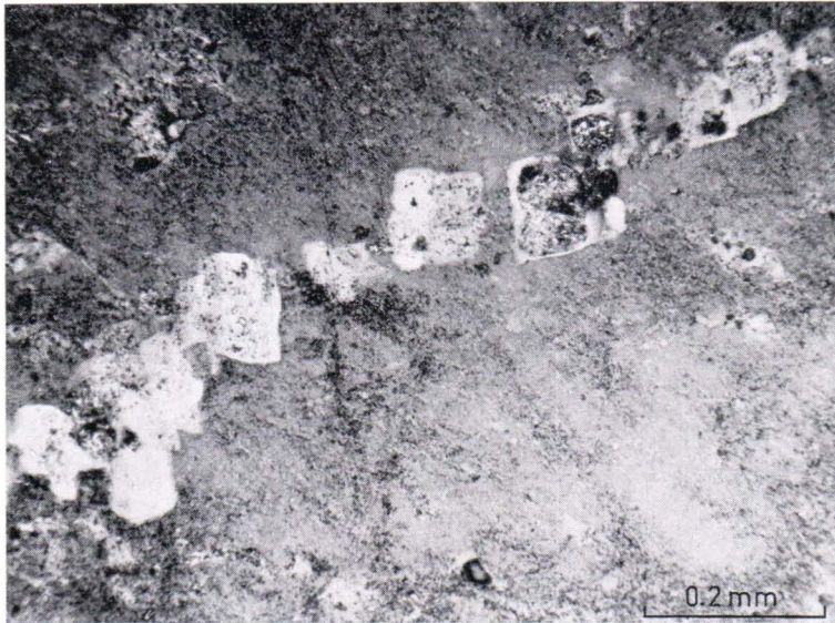
Fig. 64. Replacement vein of albitic plagioclase in perthitic microcline. The plagioclase grains show the same or nearly the same optical orientation as the perthite albite. Some of the plagioclase grains are visibly zoned. The vein continues in the adjacent quartz grain as planes of secondary fluid inclusions and as a K-feldspar vein. Even-grained type of Vakkärä granite, sample 394/PL/68.
