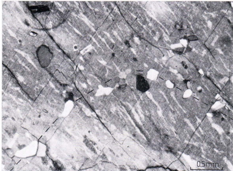
Fig. 32. Zonally arranged quartz and plagioclase inclusions in a perthitic alkali feldspar megacryst. The inclusion-rich zone is emphasized with a dotted line. Sample 37/MK/67.
