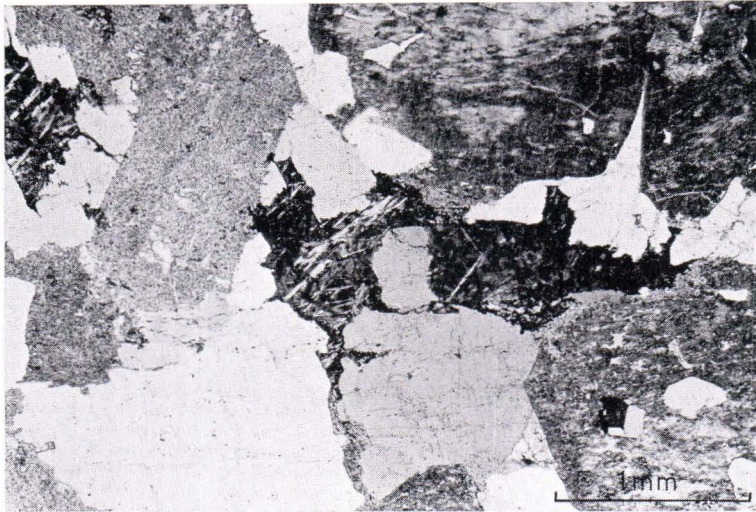
Fig. 30. Photomicrograph of the even-grained type of Väkkärä granite. An anhedral biotite aggregate between the quartz and feldspar grains. Photo E. Halme.
