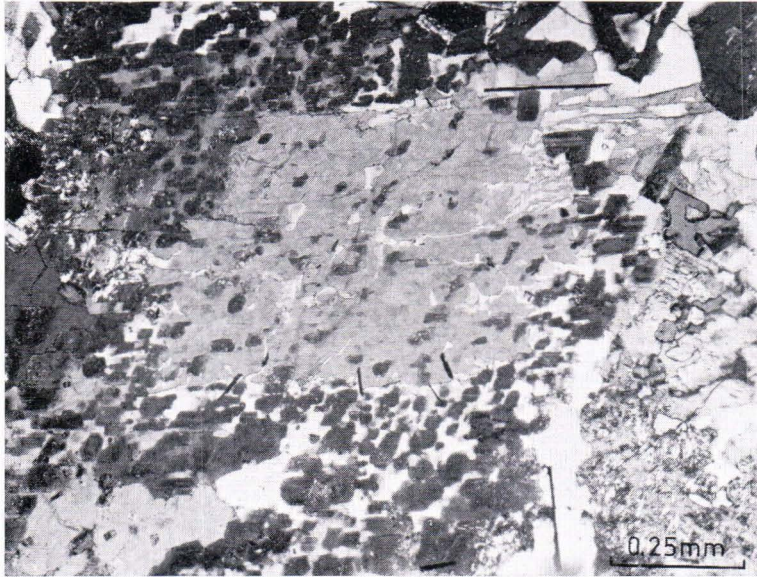
Fig. 15. Micrographic texture in Tarkki granite at the contact against a large diabase sheet. The alkali feldspar grain is surrounded by plagioclase. The quartz forms a breccia-like intergrowth with plagioclase and enters the alkali feldspar as thin veins (white). The dark blebs in the alkali feldspar are plagioclase. Sample 156/IH/67.
