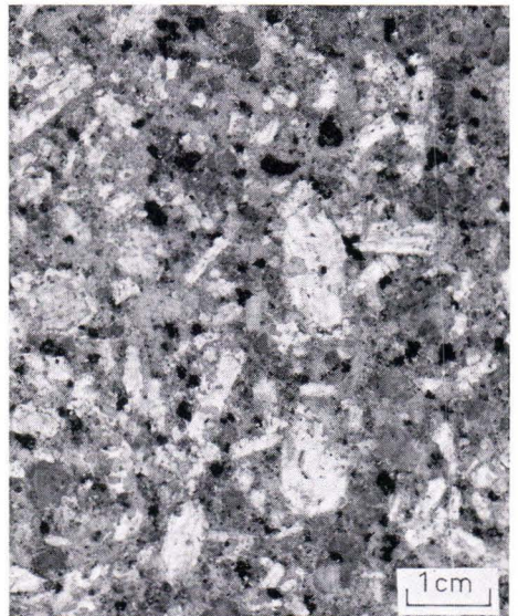
Fig. 26. Polished sample of the porphyritic type of Väkkärä granite. Sample 98/MK/687/H. Photo E. Halme.
