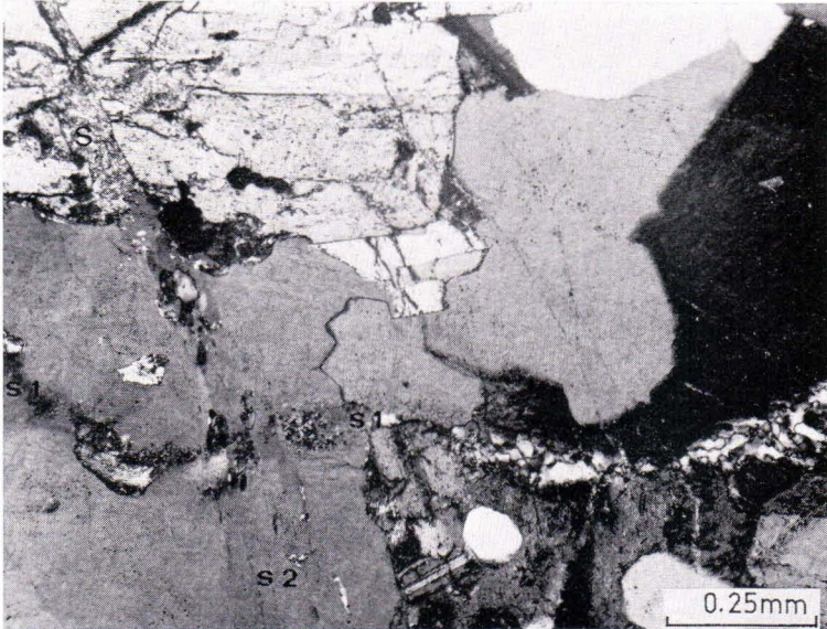
Fig. 70. In subhorizontal direction a fracture (s 1) along which silification of plagioclase and K-feldspar has taken place (see Fig. 66). This fracture is intersected by a later fracture (s 2) along which sericitization of feldspars has taken place. S sericite vein in plagioclase. The same sample as in Fig. 68.
